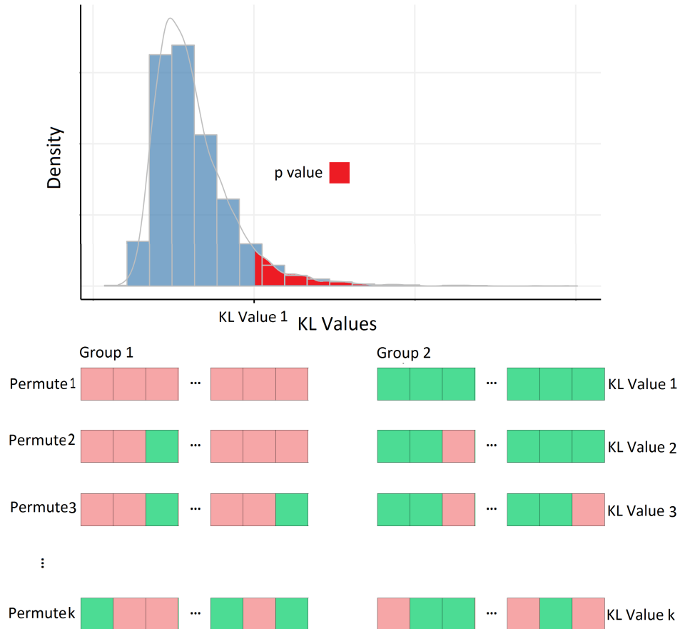
Figure 2: The significance level of KL-divergence. In order to find the significance level of a KL-divergence (KL Value 1) of a variable between two groups of samples (Permuted 1), one can permute the samples between groups for k times and compute the KL-divergence between new couple of groups (Permuted 2, Permuted 3, ..., Permuted k ). Afterward, one can find the significance level of the KL-value by considering the empirical distribution of permuted KL-values as it is illustrated in the upper plot.
