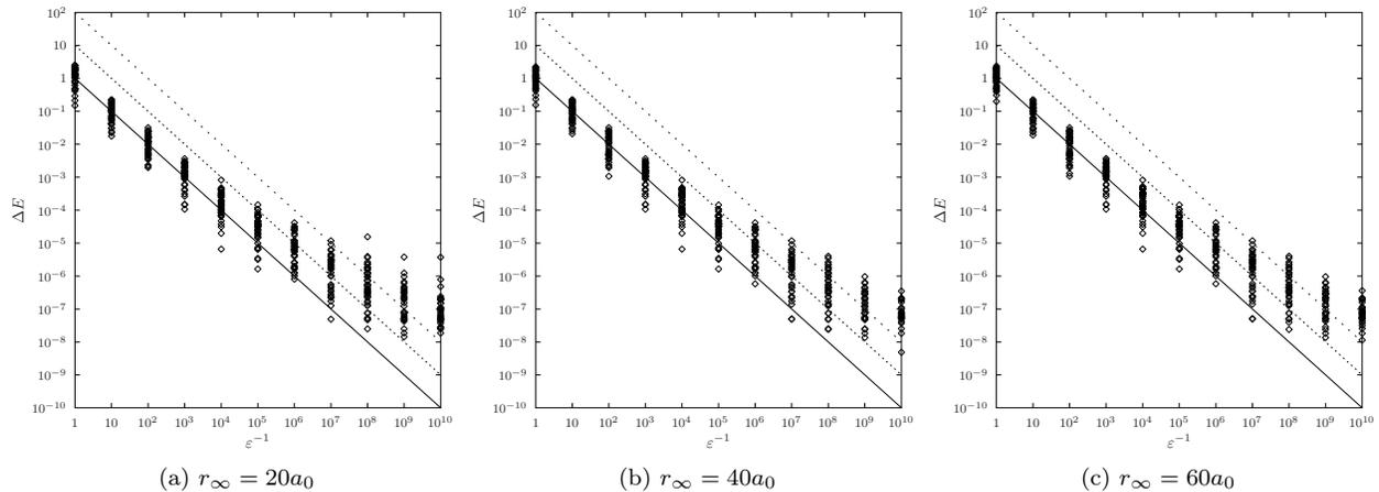
Figure 1: Convergence of the restricted HF energy for 43 first- and second-row molecules, compared to literature values from ref. 29 given in table 2. Note logarithmic scale. The ideal behavior  $\Delta E = \epsilon$  is represented by the solid line, with the dotted and loosely dotted lines illustrating behavior corresponding to  $\Delta E = 10\epsilon$  and  $\Delta E = 100\epsilon$ , correspondingly.
