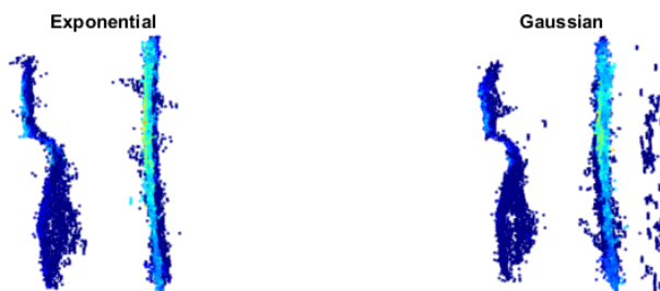
Figure 24: Recovered mannequin and back wall using a Gaussian h(t) (right) and an exponential h(t) (left). The mismatch between the true impulse response and the Gaussian one produces false returns behind the back wall.
