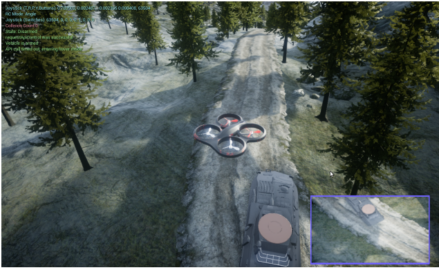
Figure 3: Screenshot of AirSim environment and landing task. Inset image in lower right corner: downward-facing camera view used for extracting the position and radius of the landing pad which is part of the observation-space that the agent learns from.
