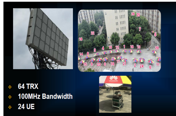
Fig. 2. The 5G base-station prototype
