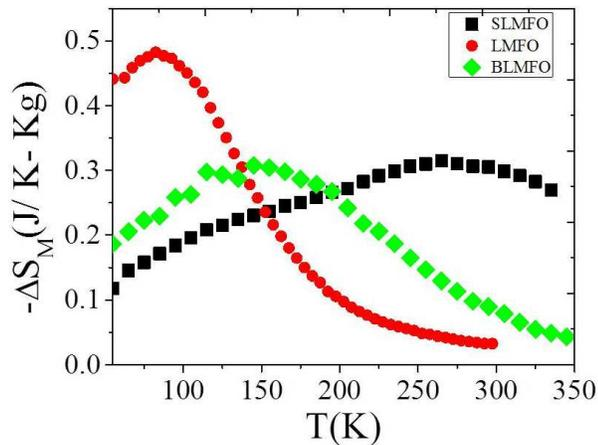
**Figure 3.** Temperature dependence of the isothermal entropy change of LMFO, BLMFO and SLMFO for a field sweep from zero to 5 T.
