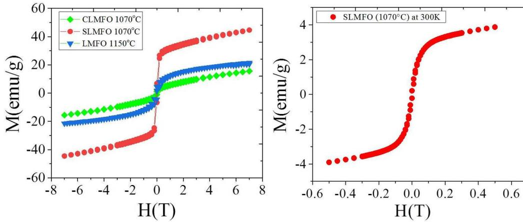
**Figure 2.** Hysteresis loops of (left) CLMFO, SLMFO and LMFO at 5 K, and (right) SLMFO at 300 K.
