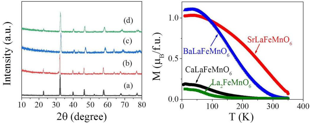
**Figure 1. (left) Powder XRD patterns of (a) LMFO, (b) BLMFO, (c) CLMFO and (d) SLMFO. (right) Magnetization as a function of temperature for LMFO and substituted LMFO samples under an applied magnetic field of 0.1T.**
