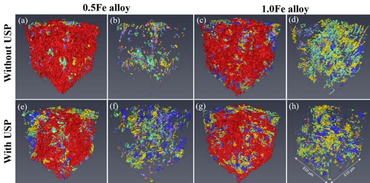
Fig. 8 3D rendered images of the Fe-rich phases in the alloys: (a-b) 0.5Fe alloy without USP; (c-d) 0.5Fe alloy with USP; (e-f) 1.0Fe alloy without USP; (g-h) 1.0Fe alloy with USP. red colour represented the interconnected particles and other colours represented the disconnected particles
