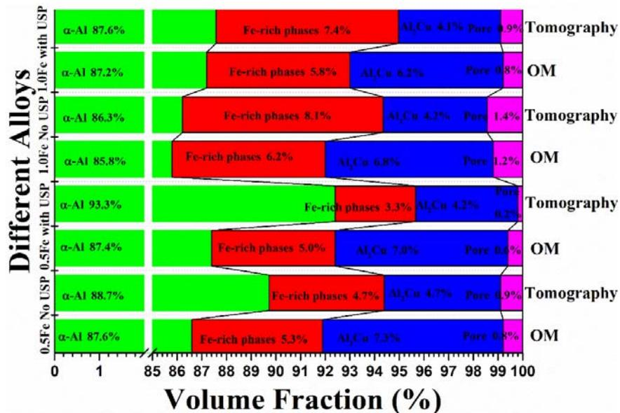
Fig. 10 Volume fractions of  $\alpha$ -Al, Fe-rich phases,  $\text{Al}_2\text{Cu}$  and pore calculated from optical microscope (OM) 2D images and synchrotron X-ray tomography.
