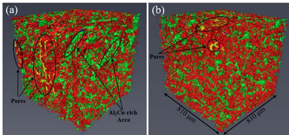
Fig. 7 Reconstructed 3D microstructures of remove the  $\alpha$ -Al matrix in the 1.0Fe alloys without USP (a) and with USP (b).
