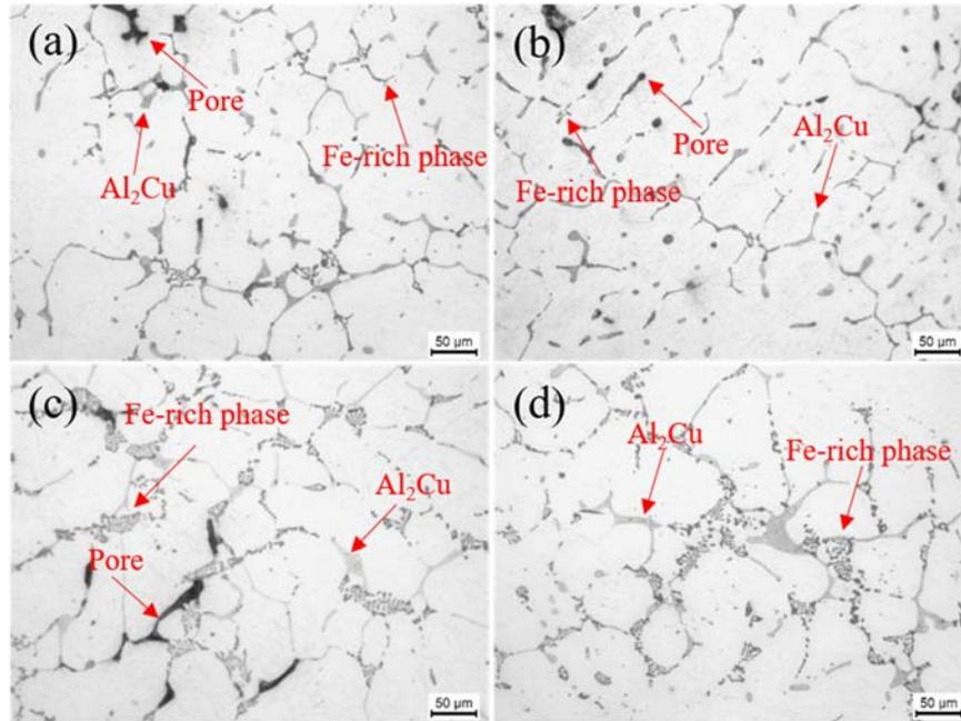
Fig. 2 Optical micrography (OM) of the microstructure: (a) 0.5Fe alloy without USP; (b) 0.5Fe alloy with USP; (c) 1.0Fe alloy without USP; (d) 1.0Fe alloy with USP.
