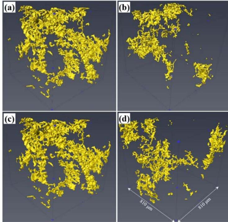
Fig. 14 Typical 3D rendered structure of pores: (a) 0.5Fe without USP; (b) 0.5Fe with USP; (c) 1.0Fe without USP; (d) 1.0Fe with USP.
