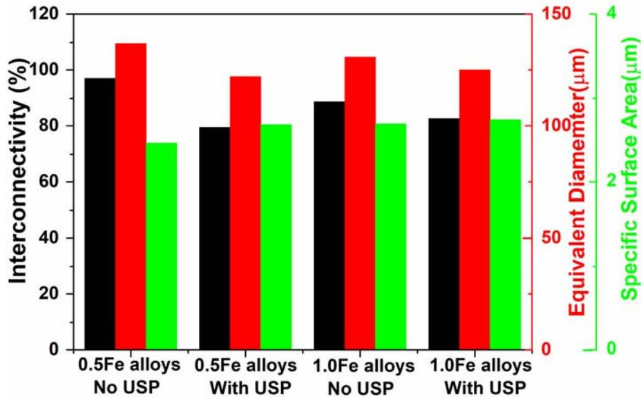
Fig. 9 Statistics of interconnectivity, equivalent diameter and specific surface area of the Fe-rich phases in the alloys with and without USP.
