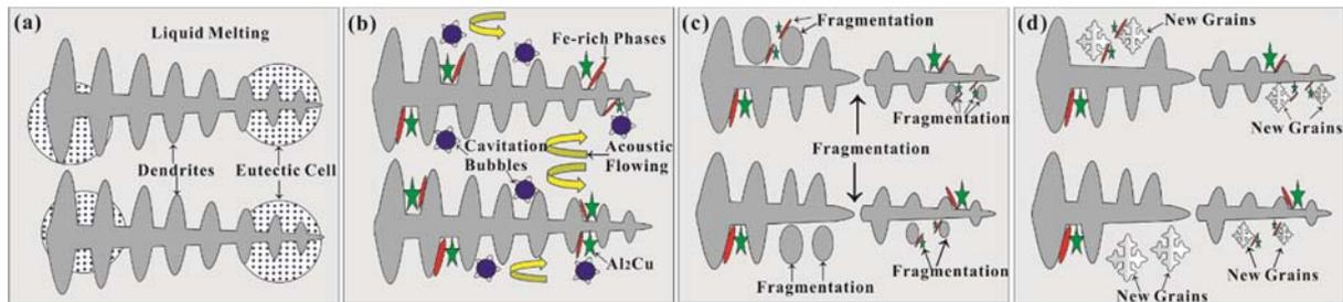
Fig. 16 Schematic diagram showing the acoustic streaming and bubbles breaking the  $\alpha$ -Al matrix and intermetallic phases induced by USP.
