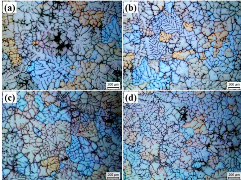
Fig. 3 Polarised light micrographs of the alloys: (a) 0.5Fe alloy without USP; (b) 0.5Fe alloy with USP; (c) 1.0Fe alloy without USP; (d) 1.0Fe alloy with USP.
