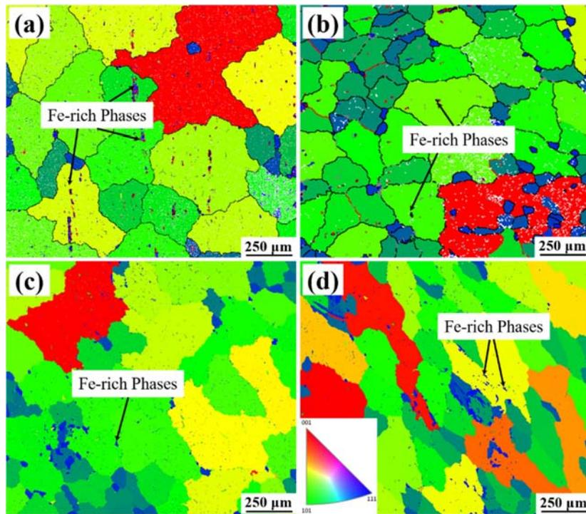
Fig. 4 EBSD shows the grain sizes of the alloys: (a) 0.5Fe alloy without USP; (b) 0.5Fe alloy with USP; (c) 1.0Fe alloy without USP; (d) 1.0Fe alloy with USP.
