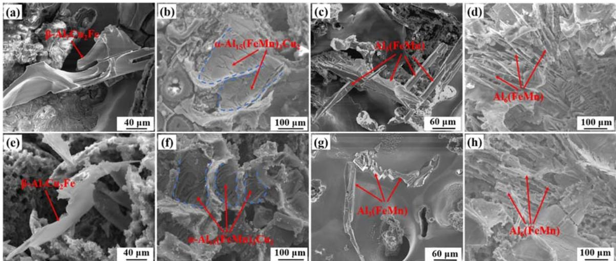
Fig. 6 The SEM images showing the deeply-etched Fe-rich phases: (a-d) without USP; (e-h) with USP; (a, e)  $\beta$ -Al<sub>7</sub>Cu<sub>2</sub>Fe; (b, f)  $\alpha$ -Al<sub>15</sub>(FeMn)<sub>3</sub>Cu<sub>2</sub>; (c, g) Al<sub>3</sub>(FeMn); (d, h) Al<sub>6</sub>(FeMn).
