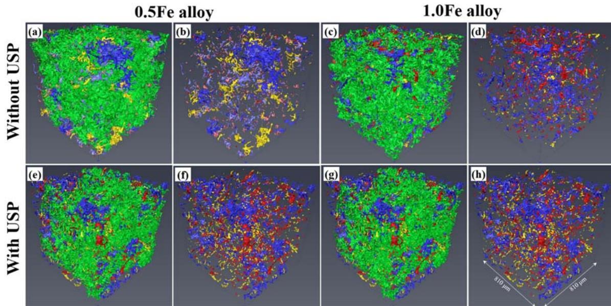
Fig. 12 Typical 3D rendered  $\text{Al}_2\text{Cu}$  phases: (a-b) 0.5Fe alloy without USP; (c-d) 0.5Fe alloy with USP; (e-f) 1.0Fe alloy without USP; (g-h) 1.0Fe alloy with USP. Green colour represented the interconnected  $\text{Al}_2\text{Cu}$  particles and other colours represented the dis-interconnected  $\text{Al}_2\text{Cu}$  particles.
