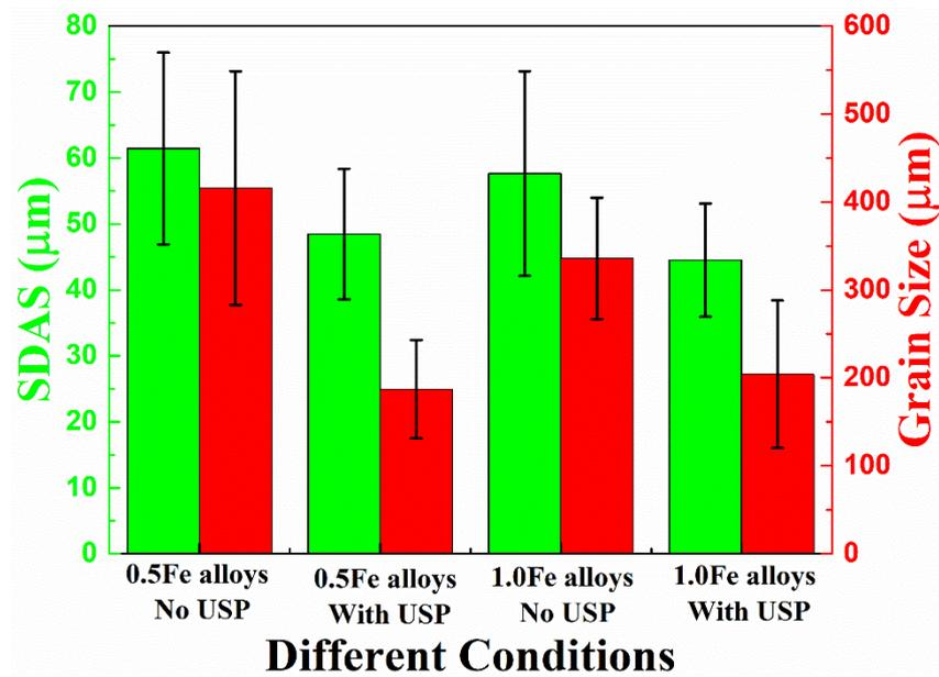
Fig. 5 Variation of secondary dendrite arm spacing (SDAS) and grain size as alloys with and without USP.
