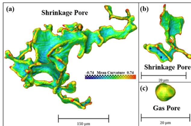
Fig. 15 The enlarged 3D morphology of pores: (a, b) shrinkage pore; (c) gas pore.
