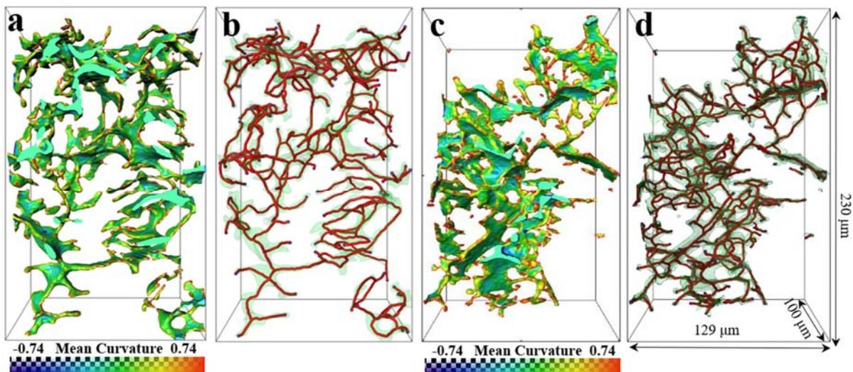
Fig. 13 The mean curvature and skeletonization of enlarged single  $\text{Al}_2\text{Cu}$  particles: (a, b) 0.5Fe alloy without USP; (c, d) 0.5Fe alloy without USP.
