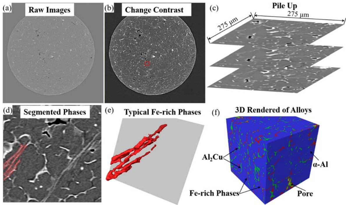
Fig. 1 Detailed image processing procedure: (a) a typical raw image from the tomography scan in 1.0Fe alloy; (b) images processed using a 3D bilateral filter; (c) pile up the images in the Avizo software; (d) segmented the phases through different threshold values; (e) a 3D rendered typical Fe-rich phases image; (f) 3D rendered different phases and pores in 1.0Fe alloy.
