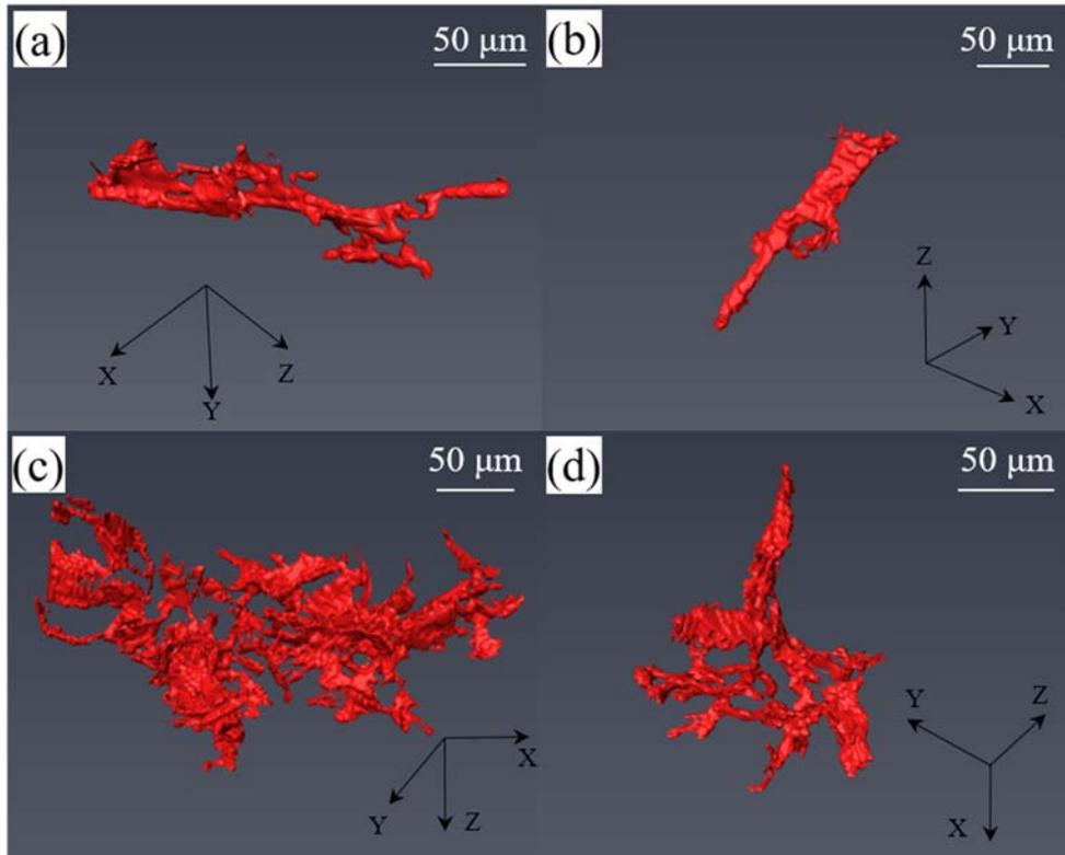
Fig. 11 Typical 3D rendered single Fe phases: (a)  $\text{Al}_3(\text{FeMn})$  without USP; (b)  $\text{Al}_3(\text{FeMn})$  with USP; (c)  $\alpha\text{-Al}_{15}(\text{FeMn})_3\text{Cu}_2$  without USP; (d)  $\alpha\text{-Al}_{15}(\text{FeMn})_3\text{Cu}_2$  with USP.
