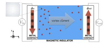
FIG. 1. A schematic for the proposed injection and detection of vortices. The electric current in the left magnetized contact pumps vortices into the insulating bulk. The applied voltage is  $V_{\rm in}$ . The vortices leaving the system through the right magnetized contact sustain the output voltage  $V_{\rm out}$ . The drag coefficient  $C_d \equiv V_{\rm out}/V_{\rm in}$  quantifies the efficiency of the topological vorticity transport.
