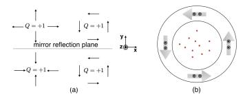
FIG. 2. Structural symmetries of the vortices and the applied torque setup: (a) Vortex charge  $\mathcal{Q}$  is invariant under the xz reflection. (b) A nonequilibrium vortex density can be controlled by the electric current circulating around the magnetic region. Red points represent vortex cores. Arrows represent electric current  $\mathbf{I} = I\hat{\mathbf{t}}$ , where the unit vector  $\hat{\mathbf{t}}$  curls anticlockwise in the metal contact that is magnetized out of the xy plane.
