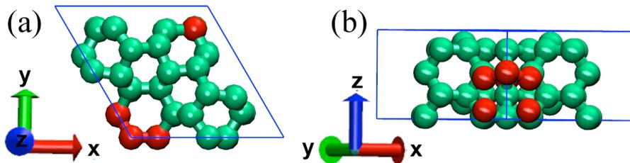
Figure 1. Unit cell of protomene: (a) top and (b) side of view. The atoms highlighted in red (darker) and green (lighter) are bonded in  $sp^2$  and  $sp^3$  hybridizations, respectively.
