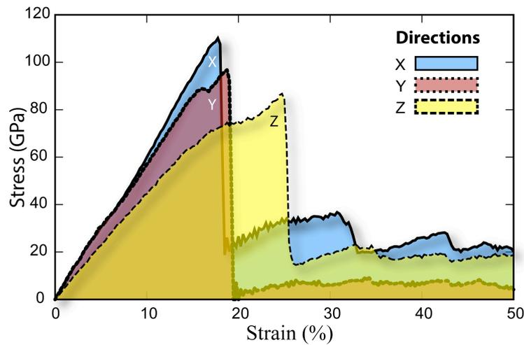
Figure 2. Stress-strain curves for protomene when a uniaxial stress applied in the x, y, and z directions.
