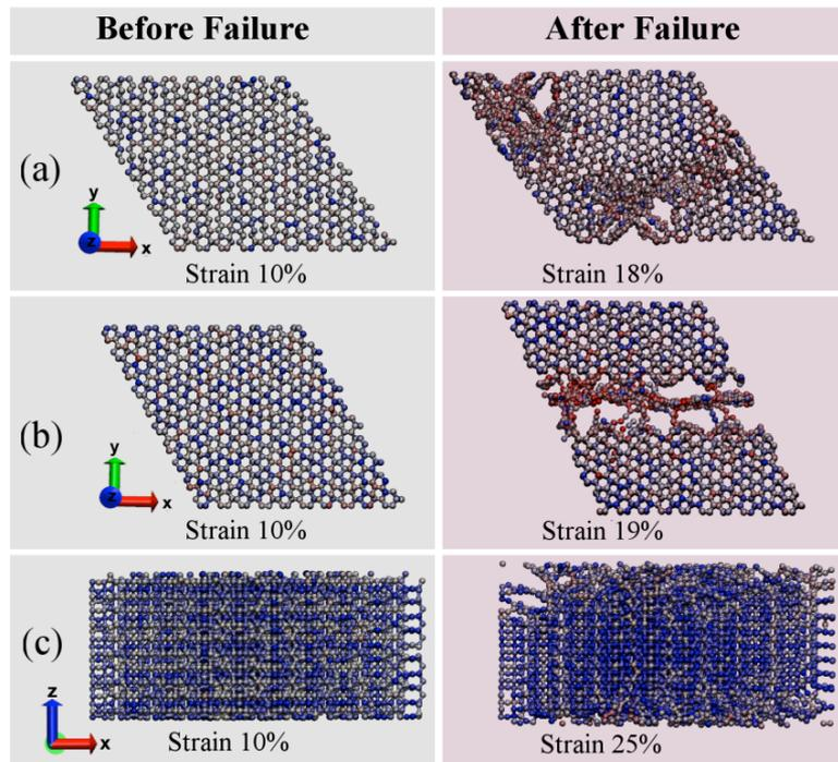
Figure 3. MD snapshots (before and after structural failure) of stress distribution in protomene for uniaxial tensile procedure along (a) x, (b) y, and (c), z directions. The atoms are colored accordingly to its von Mises stress values (vary from blue/lighter (low) to red/darker (high)).
