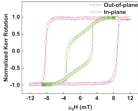
**Supplementary Figure 1 | Magneto-optic Kerr loops for the pillar of the Pt/FM1/Ta/FM2 double magnetic layered device.** The pink squares and the green circles correspond to Kerr loops measured out-of-plane and in-plane, respectively.
