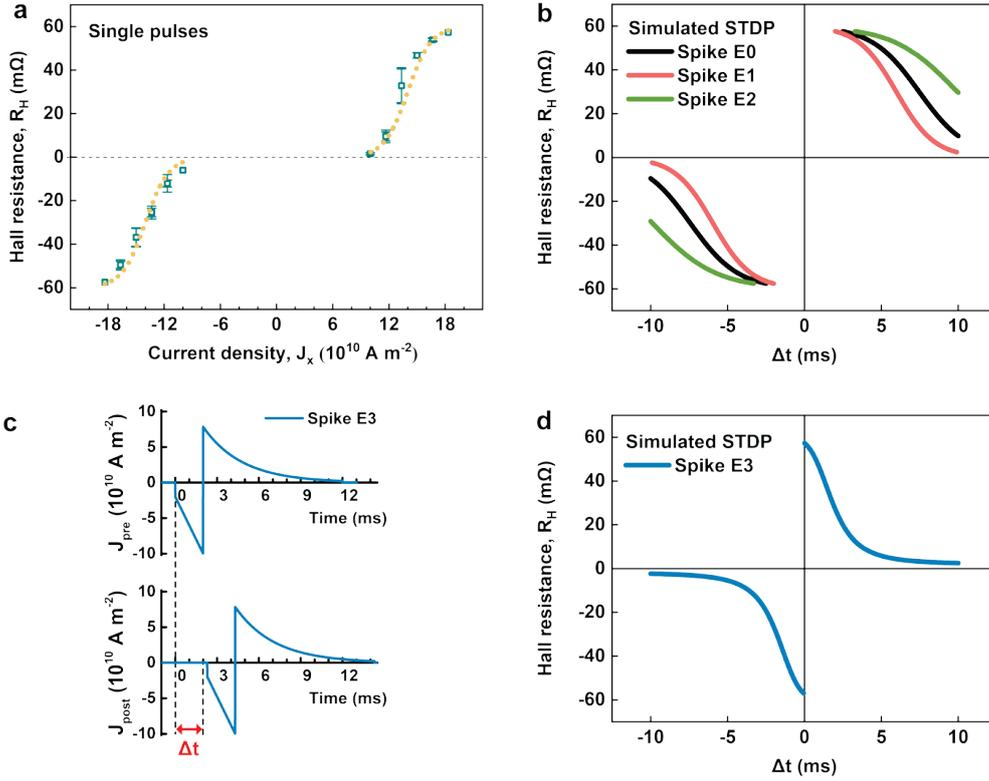
**Supplementary Figure 4 | Simulations of STDP resulting from overlapped spikes.** **a**, Fittings (yellow dotted line) of the  $R_H$  changes by single pulses in Manuscript Figure 2b. **b**, simulated STDP windows for Spike E0, E1, and E2. **c**, Spike waveform with exponentially decaying amplitude (Spike Exp). **d**, simulated STDP window for Spike Exp.
