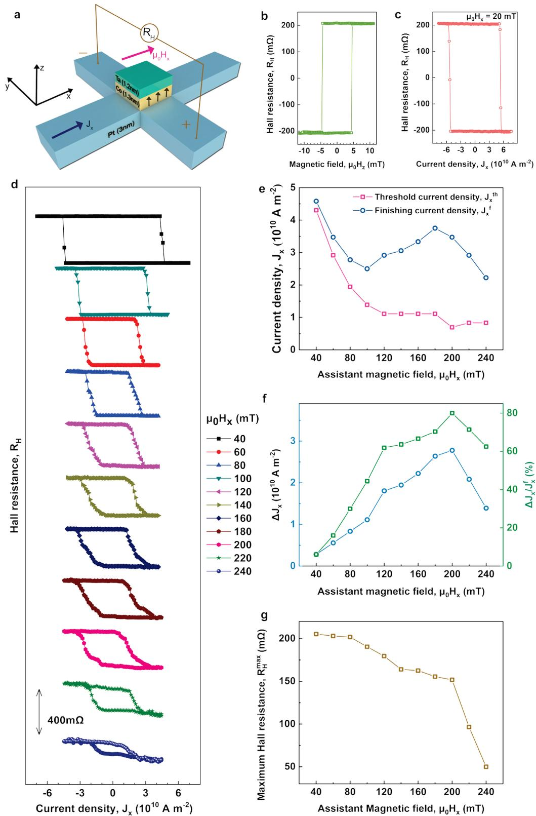
**Figure 3** SOT switching of Pt/FM1/Ta reference sample. **a**, schematic of the Pt/FM1/Ta reference device that consists of a Ta(0.5 nm)/Pt(3 nm) Hall bar with a 6  $\mu\text{m}$ -wide Co(1.3
