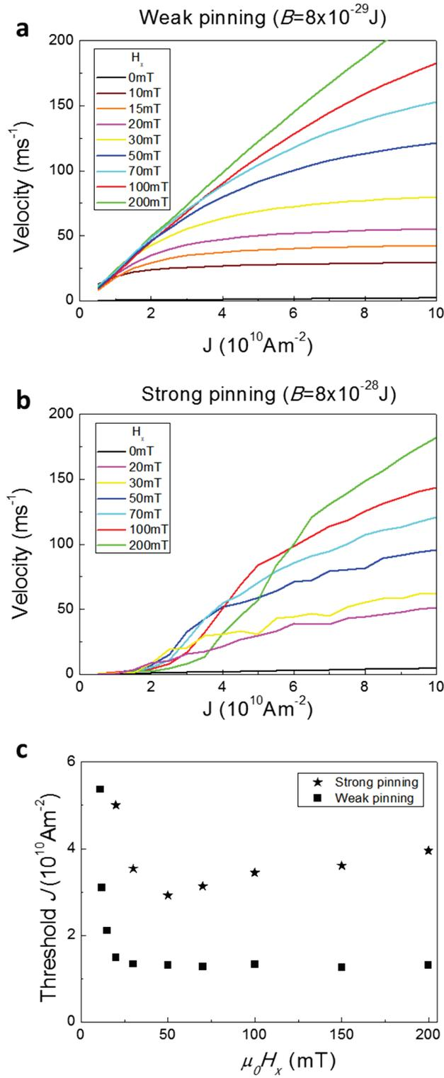
**Supplementary Figure 7 | Calculated domain wall velocity, plotted against current density,  $j$ , for various in-plane magnetic field  $\mu_0 H_x$ . Calculated velocity for **a**, weak and **b**, strong pinning potentials. **c**, the calculated threshold current density versus  $\mu_0 H_x$  for the weak and strong pinning regimes.**
