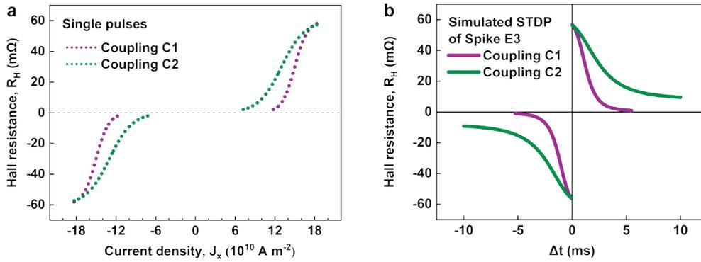
**Supplementary Figure 8 | Simulations of STDP under different functions of  $R_H$  versus single pulse's  $J_x$ .** **a**, The different given functions of  $R_H$  versus single pulse's  $J_x$  (for two corresponding supposed coupling magnitudes, C1 and C2, respectively). **b**, Simulated STDP windows for C1 and C2 with spike waveform in Supplementary Figure 4d (Spike Exp).
