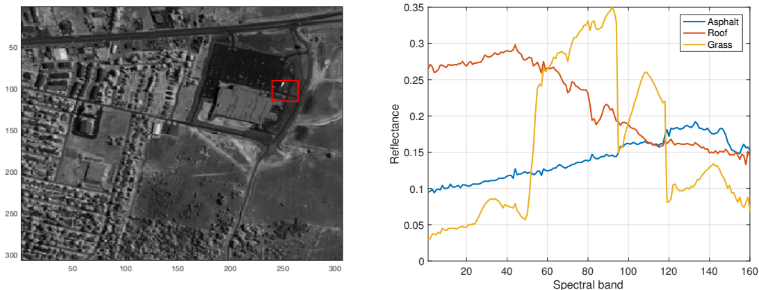
Figure 7: Urban hyperspectral image (left) and spectra of three materials present in the image (right). The data and the population spectra are obtained from http://www.escience.cn/people/feiyunZHU/Dataset_GT.html .
