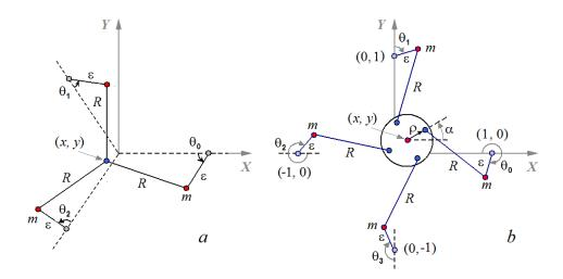
Figure 1: Hinge mechanisms based on rotators, whose angles of revolution about fixed axes are given by  $\theta_i(t)$ , with imposed holonomic constraint, which in the limiting case  $\varepsilon \ll R = 1$  reduces to the equation  $\sum_{i=0}^{N-1} \cos \theta_i = 0$ , where N=3 (a) or 4 (b).
