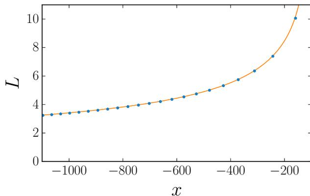
FIG. 7: Evolution of the wavelength of the nonlinear oscillations within the DSW as a function of position  $x$ . The figure corresponds to the time evolution of the parabolic initial profile represented in the lower left plot of Fig. 6 ( $t = 100$ ). The continuous line represents the results of Whitham theory and the points are the value of the wavelength extracted from the numerical simulations.
