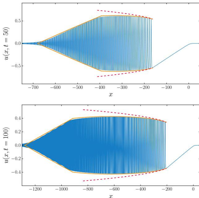
FIG. 8: Evolution of an initial square profile of type (76) with  $x_0 = 80$  after a time  $t = 50$  (upper plot) and  $t = 100$  (lower plot). The blue solid lines are the results of numerical simulations. The orange envelopes are determined by Whitham method. The red dashed envelopes are the asymptotic self-similar results obtained in Sec. IV. Note the change of scale in the axis of the two plots.
