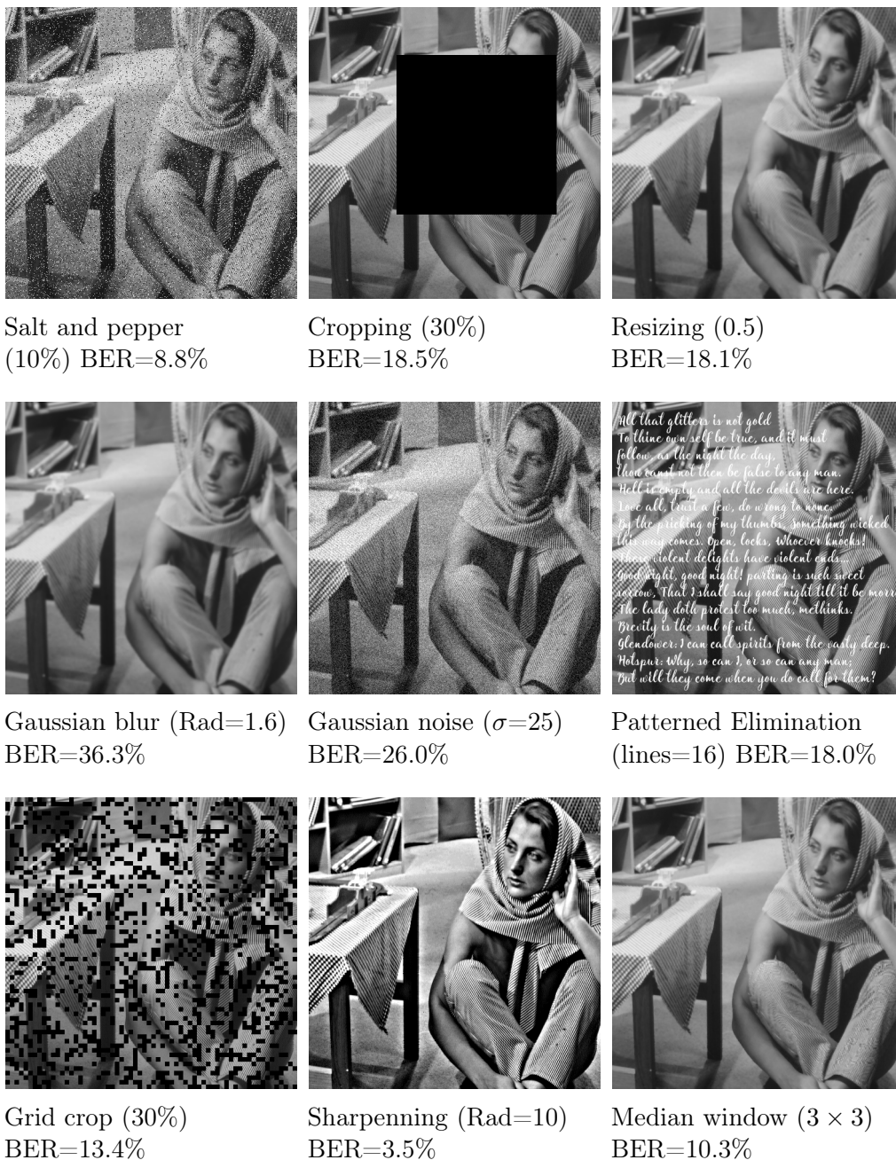
Figure 8: Visual effects of various attacks on Barbara. For each attack, the attack level/parameter and the resulting extraction BER are shown for MT-NET ( \alpha=0.6 )
