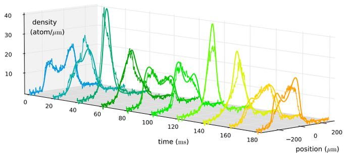
FIG. 4. Quench from double-well to harmonic potential, compared to the GHD prediction, with an atomic cloud that contains  $N \simeq 3500$  atoms initially. The main features of the experimental data are well reproduced by GHD. One experimental effect, not modeled in GHD, that appears to be particularly important, are the three-body losses: after 180 ms, the number of atoms drops by approximately 15%.
