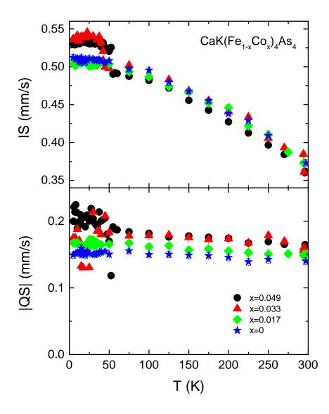
FIG. 9: (color online) Temperature dependent hyperfine parameters obtained from fits of  ${}^{57}$ Fe Mössbauer spectra of CaK(Fe<sub>1-x</sub>Ni<sub>x</sub>)<sub>4</sub>As<sub>4</sub> samples with x = 0, 0.017, 0.033, and 0.049. at different temperatures: (a) isomer shift (IS), (b) absolute value of the quadrupole splitting (|QS|). Data for CaKFe<sub>4</sub>As<sub>4</sub> are taken from Ref. [29].
