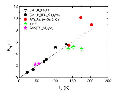
FIG. 5: (color online) The value of magnetic hyperfine field on  ${}^{57}Fe$  sites as a function of the Néel temperature for several Fe-based superconductors and related materials. Data for  $CaK(Fe_{1-x}Ni_x)_4As_4$  - this work, other points are taken from the literature.<sup>33-41</sup> Dashed line linear fit for  $(Ba_{1-x}K_x)(Fe_{1-y}Co_y)_2As_2$ .<sup>33</sup>
