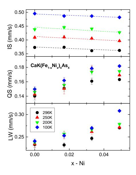
FIG. 10: (color online) Hyperfine parameters, isomer shift, (b) quadrupole splitting, and line width at selected temperatures, obtained from fits of <sup>57</sup>Fe Mössbauer spectra of  $CaK(Fe_{1-x}Ni_x)_4As_4$ samples with x = 0, 0.017, 0.033, and 0.049, plotted as a function of Ni - concentration, x. Data for CaKFe<sub>4</sub>As<sub>4</sub> are taken from Ref. [29]. Dashed lines - linear fits.
