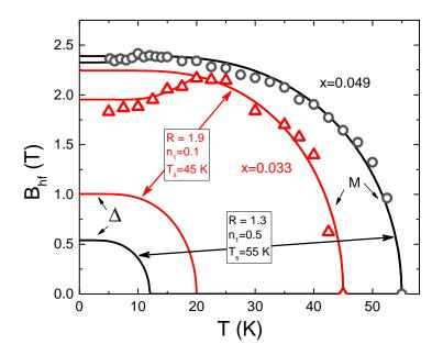
FIG. 2: (Color online) Experimental data (symbols) of  $B_{hf}(T)$  for CaK(Fe<sub>0.967</sub>Ni<sub>0.033</sub>)<sub>4</sub>As<sub>4</sub>, and CaK(Fe<sub>0.951</sub>Ni<sub>0.049</sub>)<sub>4</sub>As<sub>4</sub> overlayed with temperature dependence of scaled magnetic, M, and superconducting,  $\Delta$  order parameters (lines) from fits using model of Ref. [32] (with  $B_{hf}(T)$  serving as a proxy for magnetization). Obtained fitting parameters are listed on the plot.
