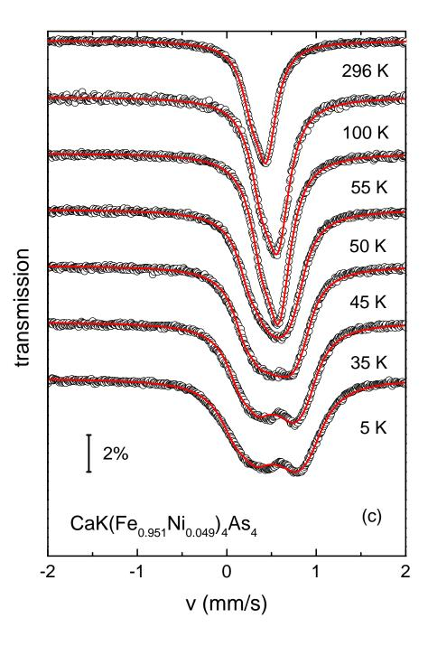
FIG. 1: (color online) <sup>57</sup>Fe Mössbauer spectra of (a)  $CaK(Fe_{0.983}Ni_{0.017})_4As_4$ , (b)  $CaK(Fe_{0.967}Ni_{0.033})_4As_4$ , and (c)  $CaK(Fe_{0.951}Ni_{0.049})_4As_4$ , at selected temperatures. Symbols - data, lines - fits.
