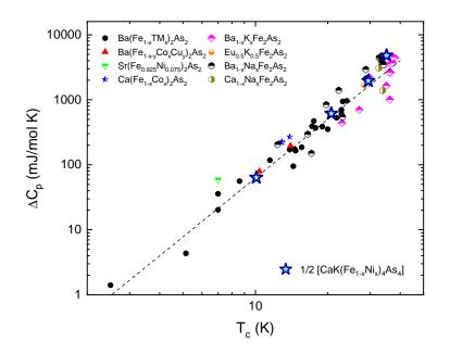
FIG. 8: (color online)  $\Delta C_p$  at the superconducting transition vs  $T_c$  for the CaK(Fe<sub>1-x</sub>Ni<sub>x</sub>)<sub>4</sub>As<sub>4</sub> samples with x = 0, 0.017, 0.033, and 0.049 plotted together with literature data<sup>46</sup> for various Fe-based superconductors. For consistency, half of the molecular weight of 1144 samples was taken for this plot. Literature data for KFe<sub>2</sub>As<sub>2</sub> and close concentrations<sup>46</sup> are not shown for simplicity.
