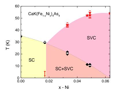
FIG. 6: (color online) x-T phase diagram for CaK(Fe<sub>1-x</sub>Ni<sub>x</sub>)<sub>4</sub>As<sub>4</sub>. Phases: SC - superconducting; SVC - magnetic spin vortex crystal, SC+SVC - coexistence of superconductivity and spin vortex crystal magnetic order. Symbols: filled - from Ref. [27], half - filled - this work: triangles and hexagons - from  $C_p(T)$ , pentagons and rhombus - from Mössbauer spectroscopy. Lines are guides for the eye.
