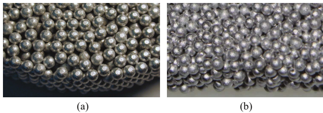
FIG. 1. (a) View of a monodisperse mesoglass sample (similar to sample H5). The sample surface has been lightly polished. (b) A polydisperse sample (sample L1). The difference in brazing between the two samples can be seen - the contacts between beads in sample L1 are generally thicker than in sample H5.
