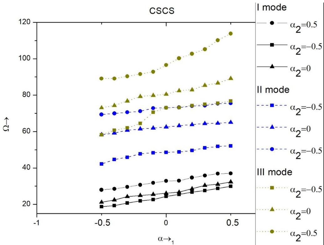
Figure 10 Frequency parameters  $\Omega$  versus non-homogeneity parameters  $\alpha_1$  for a square CSCS plate for  $\beta_1 = \beta_2 = -0.5$ , for the first, second and third mode respectively
