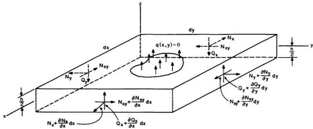
Figure 2 Force (intensity) acting on the plate element
