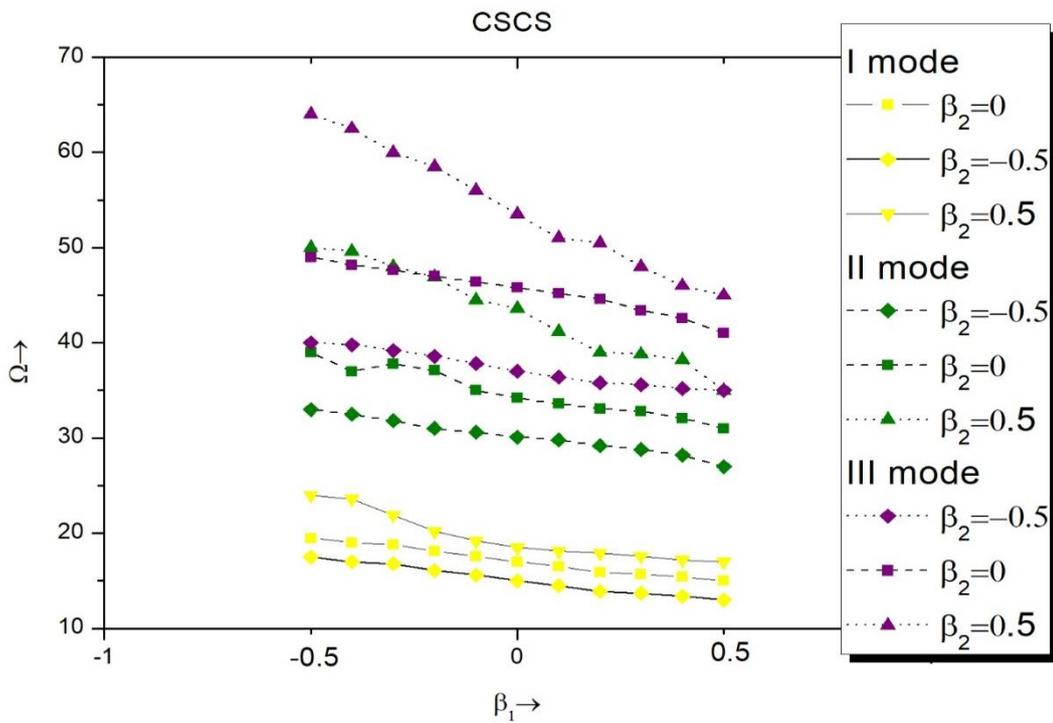
Figure 12. Frequency parameters  $\Omega$  versus non-homogeneity parameters  $\beta_1$  for a CSCS square  $\alpha_1 = \alpha_2 = -0.5$ , for the first, second and third mode respectively
