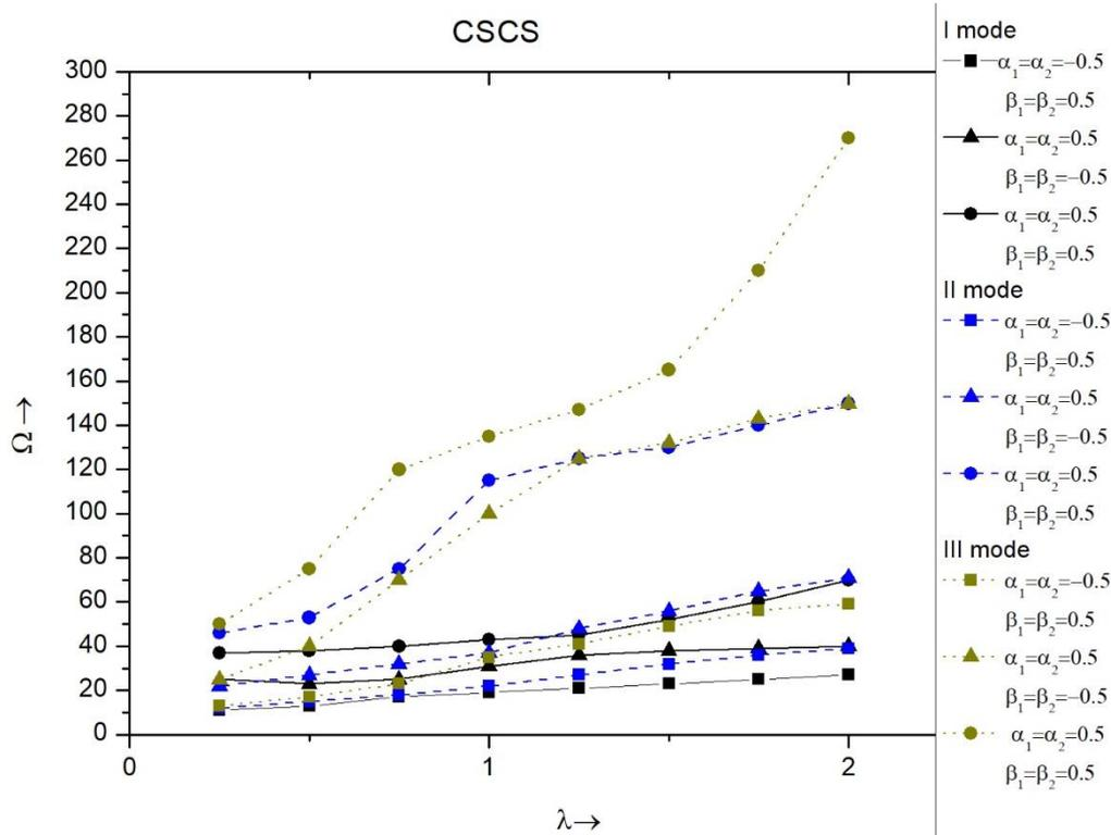
Figure 14 frequency parameters  $\Omega$  versus aspect ratio for CSCS plate
