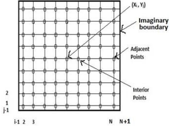
Figure 8 Demonstration of interior points, adjacent points and boundary of a rectangular plates
