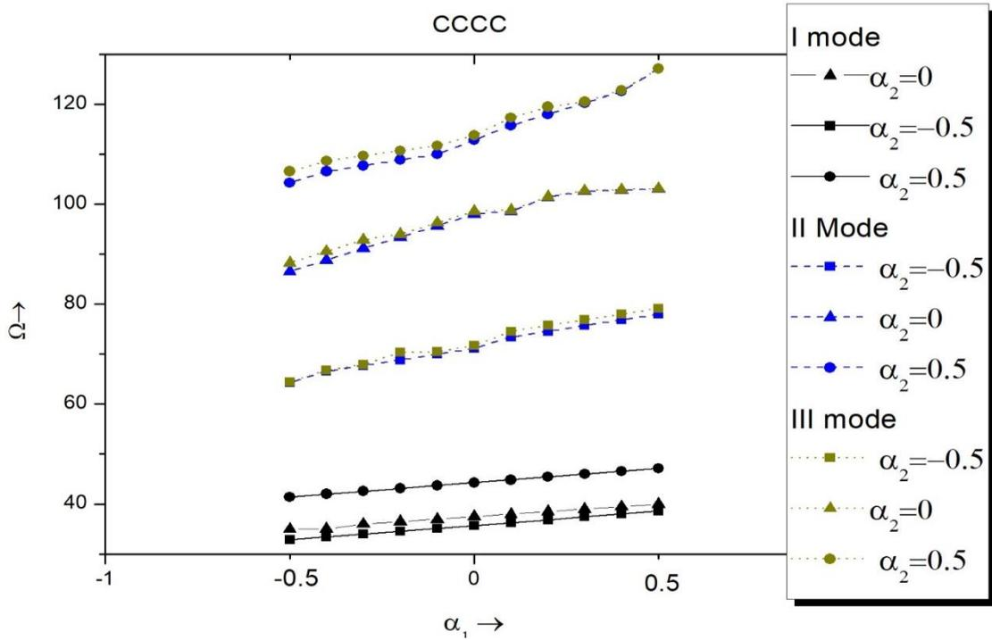
Figure 9 Frequency parameters  $\Omega$  versus non-homogeneity parameters  $\alpha_1$  for a square CCCC plate for  $\beta_1 = \beta_2 = -0.5$ , for the first, second and third mode respectively
