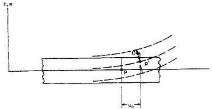
Figure 5 Kinematics of plate deformation
