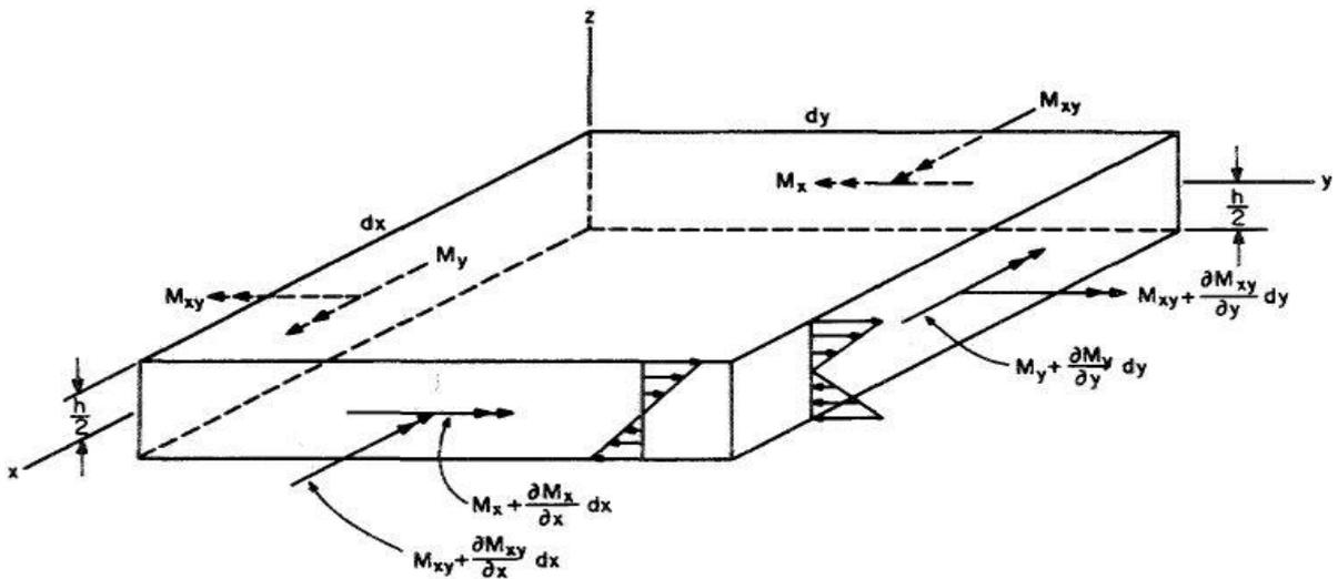
Figure 3 Moment (intensity) acting on the plate element
