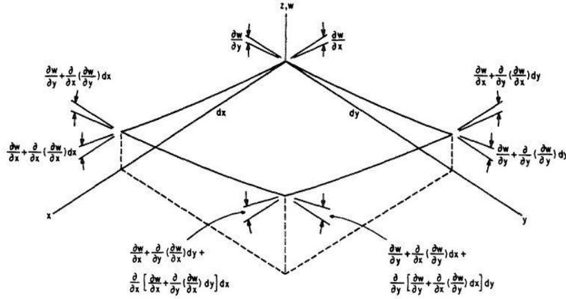
Figure 4 shows the deformed middle surface of the plate element showing slopes and their change. The figure 4 shows that incremental changes are shown at all the corner of the element with positive changes assume in positive direction. For small displacement, it is assumed that the slope and the sine of the angle are equivalent.
