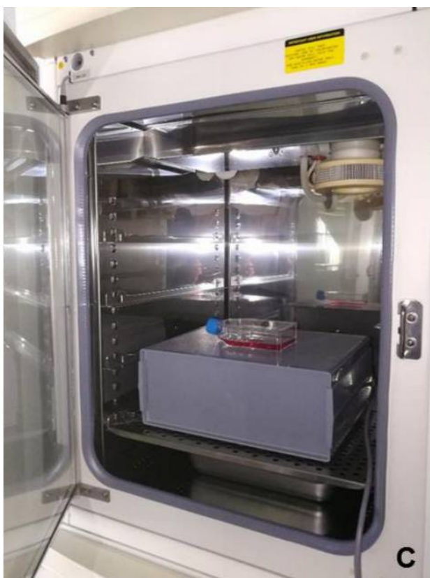
Fig. 18 - Photo of the antenna enclosure housed inside a 37°C, CO 2 controlled incubator for experiments.
