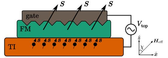
FIG. 1. Proposed experimental setup. Non-homogeneous in-plane electric field components are created by an *ac* top-gate voltage  $V_{\text{top}}$  that induce a strong diffusive spin-orbit torque (4) of the damping-like symmetry. An effective magnetic field  $\mathbf{H}$  is directed at the angle  $\chi$  with respect to  $\hat{z}$ .
