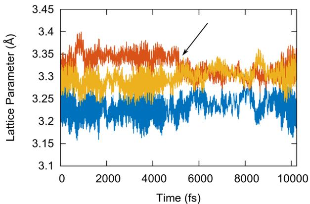
FIG. 5: A 10 ps aiMD trajectory of Ti-31.25Ta at 500 K. The arrow points out the instant at which the MT takes place.
