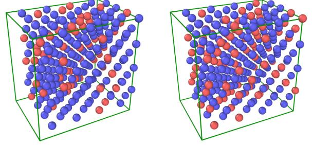
FIG. 1: The SQS employed for the simulations of Ti-25Ta (**left**) and Ti-31.25Ta (**right**). Ti atoms are blue, and Ta atoms are red.
