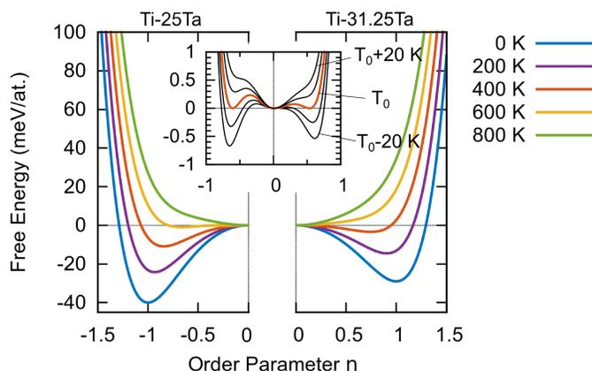
FIG. 4: The free energy profiles as a function of the order parameter for Ti-25Ta (left) and Ti-31.25Ta (right) for different temperatures. The inset shows the same profiles for an interval of temperatures around the transition temperature  $T_0$ .
