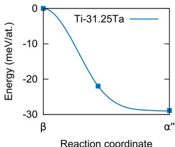
FIG. 2: Minimum energy path at 0 K for the MT between austenite ( $\beta$ ) and martensite ( $\alpha''$ ) for Ti-31.25Ta.
