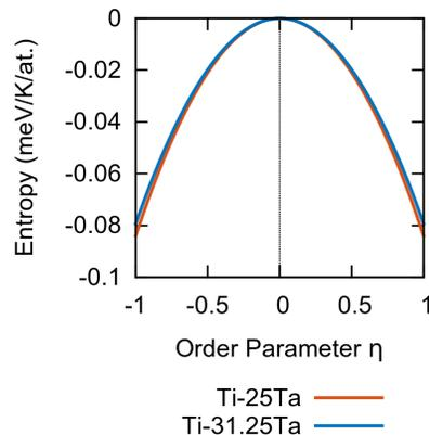
FIG. 4: Entropy as a function of the order parameter for Ti-25Ta (red) and Ti-31.25Ta (blue) obtained from the Landau-Falk expansion.
