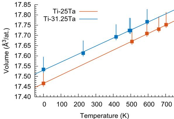
FIG. 6: The atomic volume as a function of temperature for Ti-25Ta (red) and Ti-31.25Ta (blue). The asymmetric error bars take into account the Pulay stresses.
