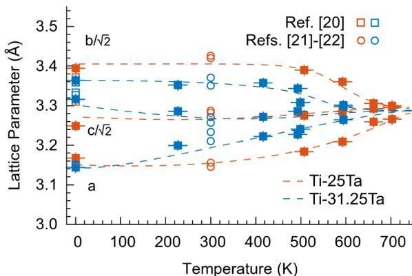
FIG. 2: Lattice parameters of Ti-25Ta (red) and Ti-31.25Ta (blue) as a function of temperature. Circles are experimental data on bulk samples and thin films at room temperature. Empty squares are DFT calculations from Ref. [20]. Broken lines are guide-to-the-eye.
