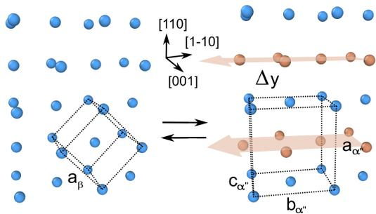
FIG. 1: The MT in Ti-Ta. The austenitic phase (left) is a bcc structure. The martensitic phase (right) is orthorhombic, and it is obtained from the austenitic phase by cell distortion and gliding of alternating  $\{110\}$  planes (in brown) along the  $\langle -110 \rangle$  direction, described by the parameter  $\Delta y$ .
