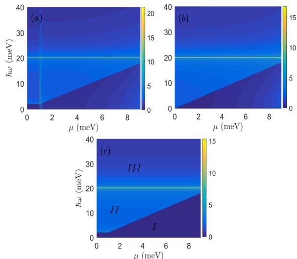
FIG. 4. Gradient plot of  $yy$ -components of conductivity (in units of  $e^2/\hbar$ ) for (a)  $m_0 = 1$  meV, (b)  $m_0 = 0$  meV, and (c) JDOS. The giant optical conductivity is only excited by frequency  $\hbar\omega = \sqrt{m_0^2 + \delta_0^2}$ .
