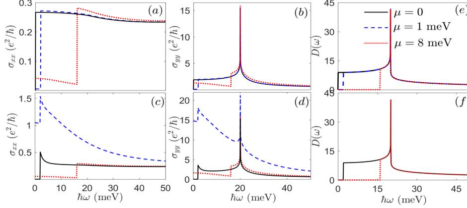
FIG. 3. Plots of the real part of  $\sigma_{xx}(\omega)$  and  $\sigma_{yy}(\omega)$  for gap-less system (Sec. (a) and (b)) and gapped system (Sec. (c) and (d)) with the corresponding JDOS in Sec. (e) (for gap-less system) and (f) (for gapped system). As shown in legend of Sec. (e), solid black curve, dashed blue and dotted red curve corresponds to  $\mu = 0$ ,  $\mu = 1$  meV and  $\mu = 8$  meV, respectively for all plots.
