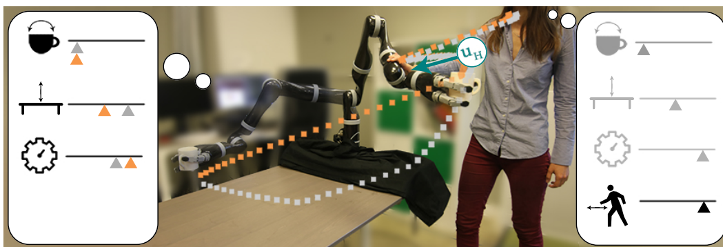
Figure 1: The human pushes the robot to indicate she wants it to stay farther away from her, but this objective falls outside the robot’s hypothesis space (i.e. robot does not reason about distance from humans). The robot detects a change in the distance to the table and erroneously learns to move closer to it (gray trajectory). Instead, with our method, the robot realizes that the human’s correction does not make sense if what she wanted was a smaller distance to the table, and it does not erroneously learn from the physical interaction (orange trajectory).
