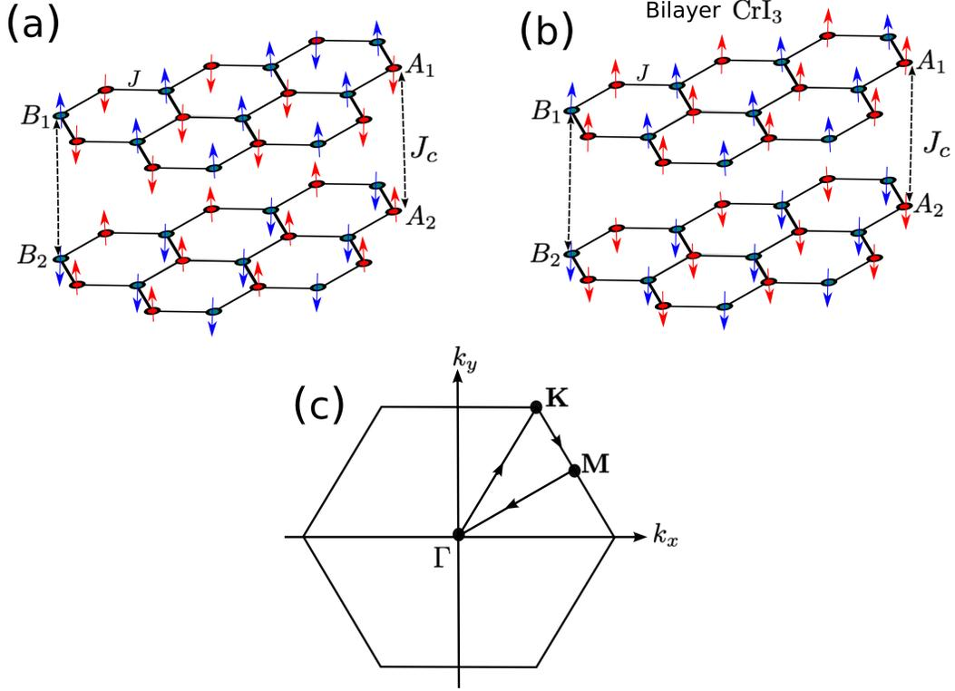
FIG. 1: Color online. (a) Bilayer honeycomb-lattice antiferromagnets coupled antiferromagnetically. (b) Bilayer honeycomb-lattice ferromagnets coupled antiferromagnetically as realized in bilayer CrI<sub>3</sub>. (c) The Brillouin zone (BZ) of the honeycomb lattice with high-symmetry paths.
