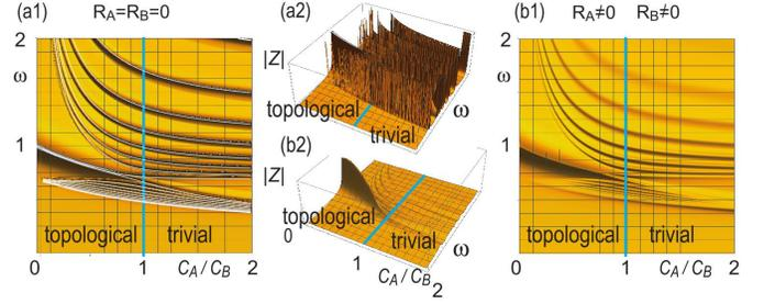
FIG. 5: Impedance peaks are shown in the  $(C_A/C_B)$ - $\omega$  plane. Phase transition occurs at  $C_A = C_B$ . (a) Many impedance peaks are generated as implied by Eq.(8) both in the topological and trivial phases of the Hermitian SSH model ( $R_A = R_B = 0$ ). White curves represent the analytical result (8). (b) All these peaks are suppressed drastically except for the topological peak in the topological phase of the reciprocal non-Hermitian SSH model ( $R_A \neq 0, R_B \neq 0$ ).
