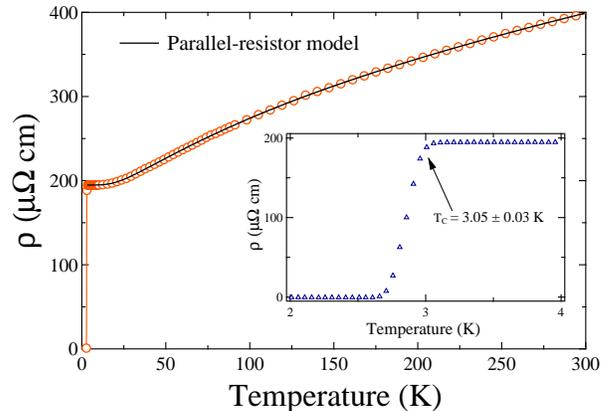
FIG. 2. Temperature dependence of resistivity in the range  $1.8 \text{ K} \leq T \leq 300 \text{ K}$ . The inset shows the drop in resistivity at the superconducting transition,  $T_C = 3.05 \pm 0.03 \text{ K}$ . The normal state resistivity fitted with the parallel-resistor model in the temperature range  $5 \text{ K} \leq T \leq 300 \text{ K}$ .
