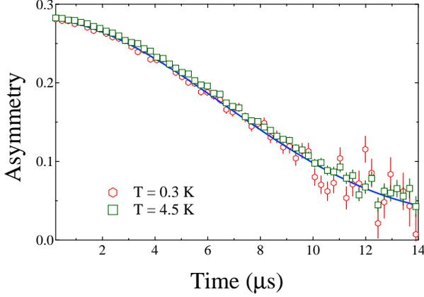
FIG. 6. ZF -  $\mu$ SR spectra collected above ( $T = 4.5$  K) and below ( $T=0.3$  K) the transition temperature. The solid line is fit to Eq. 19.
