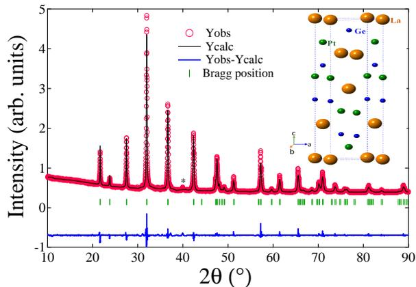
FIG. 1. Powder x-ray diffraction pattern for LaPtGe sample obtained at room temperature using Cu  $K_{\alpha}$  radiation (red line). The black solid line shows the Rietveld refinement whereas the blue line shows the difference between observed and calculated one. The inset shows the crystal structure.
