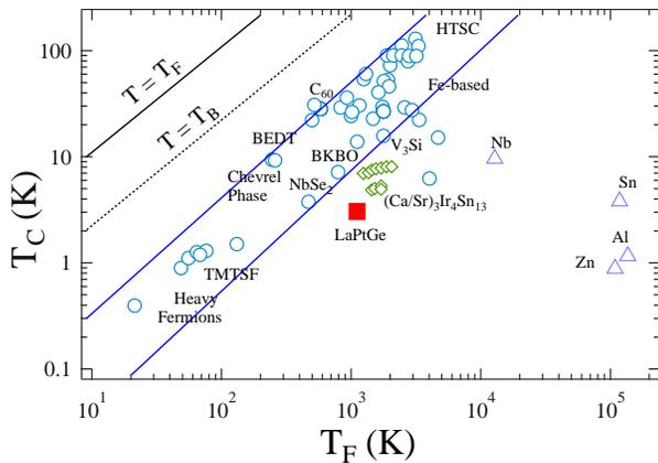
FIG. 9. The Uemura plot showing the superconducting transition temperature  $T_c$  vs the effective Fermi temperature  $T_F$ , where LaPtGe is shown as a solid red marker. Other data points plotted between the blue solid lines is the different families of unconventional superconductors [49, 50].
