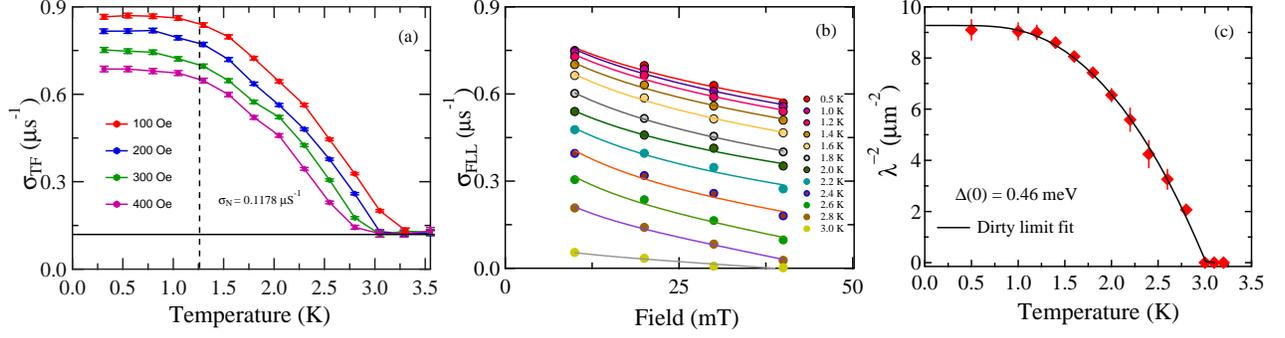
FIG. 8. (a) Temperature dependence of TF -  $\mu$ SR depolarisation rate collected at different fields. (b) Isothermal field dependence of depolarisation. (c) Temperature dependence of inverse magnetic penetration depth square. Solid line is the fit to the s-wave model.
