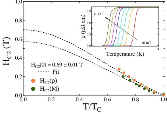
FIG. 4. Temperature dependence of upper critical field  $H_{C2}$  determined via magnetization and resistivity measurements. The solid lines are fit to the data using Eq. 5. The inset shows the resistivity curves at different applied magnetic fields.
