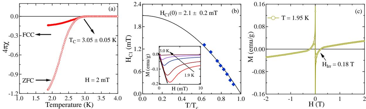
FIG. 3. (a) Temperature dependence of magnetic moment collected via zero field cooled warming (ZFCW) and field cooled cooling (FCC) methods under applied field of 2 mT. (b) Temperature dependence of lower critical field  $H_{C2}$ . The inset shows the low field magnetization data at different temperatures. (c) Magnetization data collected at 1.95 K in the range  $-2 \text{ T} \leq H \leq +2 \text{ T}$  showing an irreversible field  $H_{\text{Irr}} = 0.18 \text{ mT}$ .
