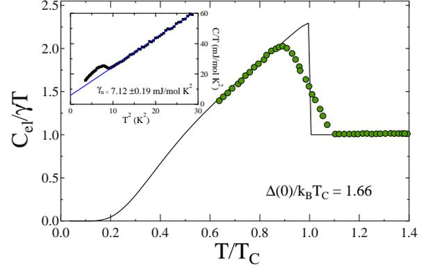
FIG. 5. Temperature dependence of electronic specific heat fitting with isotropic BCS expression (Eq. 17). The inset shows the  $C/T$  vs  $T^2$  data fit to Eq. 10.
