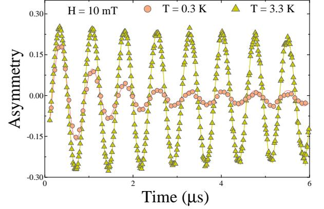
FIG. 7. TF -  $\mu$ SR signals collected above ( $T = 3.3$  K) and below ( $T = 0.3$  K) the transition temperature in an applied magnetic field of 10 mT. Fast decay of signal below  $T_C$  indicate the vortex formation.
