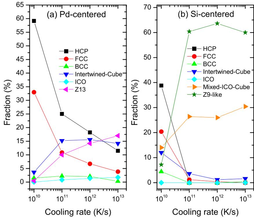
Fig. 7. The fractions of various SROs in  $\text{Pd}_{0.95}\text{Si}_{0.05}$  at  $T=300\text{K}$  as the function of cooling rate. (a) Pd-centered SROs. (b) Si-centered SROs. Our results clearly exhibit the competition between glass-forming motifs (Z13, Z9-like and Mixed-ICO-Cube) and crystalline motifs (HCP and FCC).
