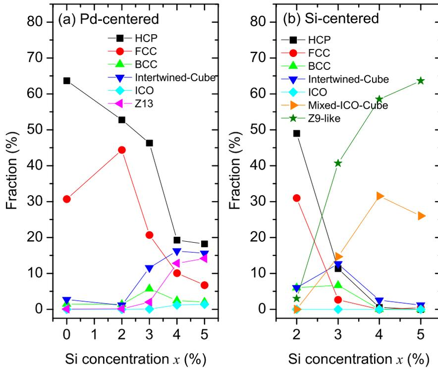
Fig. 5. The fractions of various SROs in  $\text{Pd}_{1-x}\text{Si}_x$  at  $T=300\text{K}$  by cooling at the rate of  $10^{12}$  K/s as the function of Si-doping concentration  $x$ . (a) Pd-centered SROs. (b) Si-centered SROs. It can be seen that a small amount of Si solutes would significantly suppress the crystallization of Pd and increase the fraction of glass-forming SROs (Z13, Z9-like and Mixed-ICO-Cube) in the samples, leading to the enhancement of GFA.
