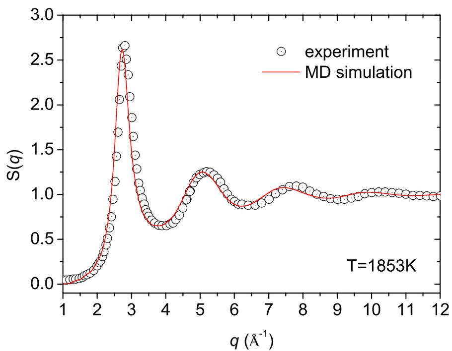
Fig. 1. The comparison of total structure factors for liquid Pd at  $T=1853\text{K}$  from MD simulation to experimental data. The red line is the result of MD simulation with semi-empirical Pd-Si EAM potential.
