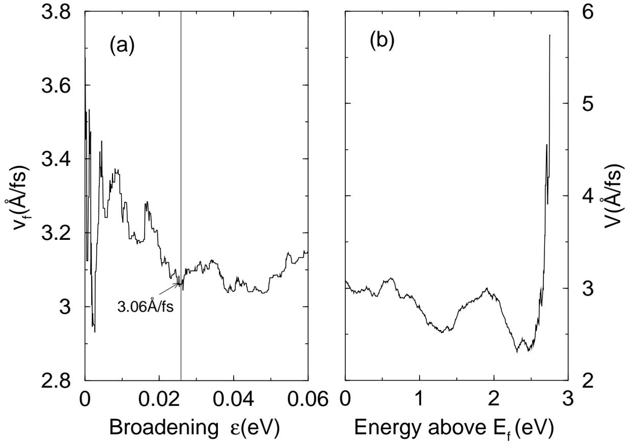
FIG. 5. (a) Fermi velocity as a function of the broadening  $\epsilon$  in the Fe/W(110) thin film. The vertical line denotes the room temperature, where we find the Fermi velocity is  $3.06 \text{ \AA/fs}$ . This is higher than that in Ni. (b) Velocity as a function of the energy with respect to the Fermi energy. We include an energy window of  $0.2 \text{ eV}$ . We only plot the energy up to  $3 \text{ eV}$ .
