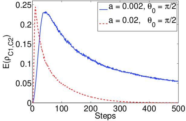
**FIG. 16.** Entanglement between the particles of coin Hilbert space in two-particle accelerated quantum walk with temporal disorder (ATQW) for different value of  $a$ . Initial state is  $|\psi_{in}\rangle = |\uparrow\uparrow\rangle \otimes |x=0\rangle$  averaged over 1000- runs. For larger  $a$  entanglement dies faster in time.
