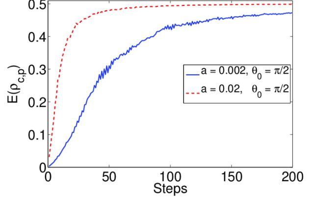
**FIG. 17.** Entanglement between the coin and position Hilbert space in two-particle accelerated quantum walk with temporal disorder (ATQW) as function of time (steps) for different value of  $a$ . Initial state is  $|\psi_{in}\rangle = |\uparrow\uparrow\rangle \otimes |x=0\rangle$  averaged over 500- runs. For larger  $a$  entanglement reaches maximum value faster in time.
