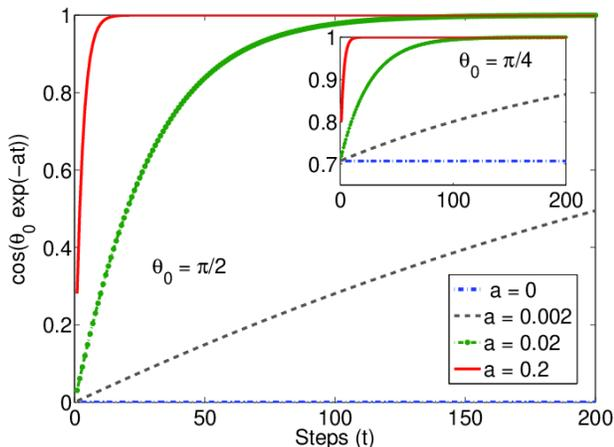
**FIG. 1.** Effect of parameter  $a$  which induces acceleration on the quantum walker as function of  $t$  is shown by plotting  $\cos(\theta_0 e^{-at})$ . For higher value of  $a$  we can see a value reaching unity at earlier time. This gives us a range of values  $a$  to look into to understand the effect of acceleration on the quantum walk dynamics.
