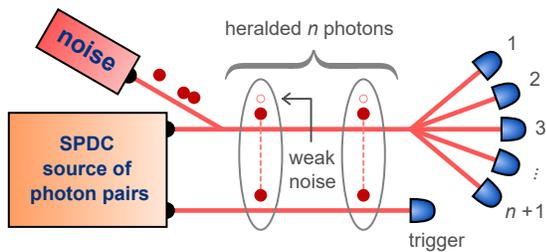
FIG. 3: Schematics of the experiment. A number of down-converted heralded photons with weak multiphoton contributions are incident on a balanced multi-channel detector consisting of single-photon avalanche diodes (SPAD). The multiphoton contribution consists of multi-pair generation and, primarily, of Poissonian noise added by coupling a laser diode to the signal. Only time windows conditioned by a trigger detection are considered, and  $n$  successive time windows are merged together.
