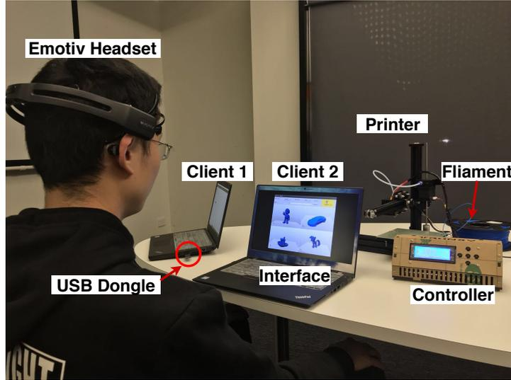
Figure 8: Online testing scenario. The user’s EEG signals are collected by Emotiv headset for recognition. The correspond object will be printed through the 3D printer.
