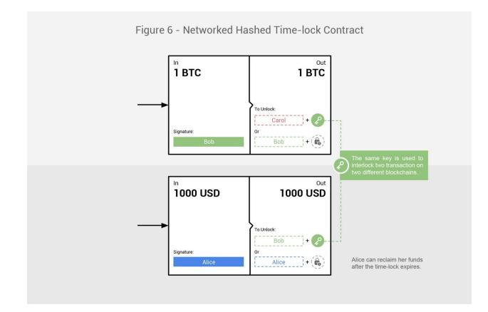
The time-lock mechanism is used as a refund mechanism in case of an intermittent routing failure. The time-locks need to be stacked from receiver towards sender to make sure no-one is able to cheat.
