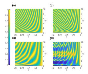
FIG. 7. Surface plot of the transmission probability as a function of E and  $\phi$  for  $V(\xi) = 20$  meV in  $R_2$  and  $R_4$  regions and in  $R_3$  (a) n = 6 with  $\theta = \pi/2$ ; (b) n = 12 with  $\theta = \pi/2$ ; (c) n = 6 with  $\theta = \pi$  and (d) n = 12 with  $\theta = \pi$ , and  $m^* = 0.173m_0$ ,  $m^* = m_0$ , otherwise.
