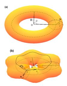
FIG. 1. (a) schematic of a torus with  $r_0 = (r_{x_0}, r_{y_0}, r_{z_0})$ ; (b) schematic of a corrugated torus described by  $r = (r_x, r_y, r_z)$  with n = 6. Here, R and  $\phi$  are the large radius and azimuthal angle, and r and  $\theta$  are the small radius and polar angle.
