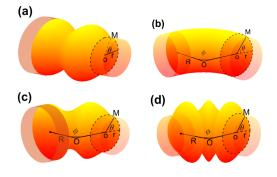
FIG. 2. (a) schematic of a deformed tube; (b) schematic of a quarter torus; (c) schematic of a quarter corrugated torus with n = 6; (d) schematic of a quarter corrugated torus with n = 12.
