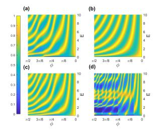
FIG. 5. Transmission probability versus incident energy E and azimuthal angle  $\phi$  for the model with  $V(\xi) = 20$  meV in  $R_2$  and  $R_4$ , and for (a)  $V_g(\xi)$  given by a corrugated tube; (b)  $V_g(\xi)$  induced by a quarter torus; (c)  $V_g(\xi)$  provided by a quarter torus with 1.5 corrugations; (d)  $V_g(\xi)$  provided by a quarter torus with three corrugations, and  $m^* = 0.173m_0$  and  $\theta = \pi$  in  $R_3$ ,  $m^* = m_0$ , otherwise.
