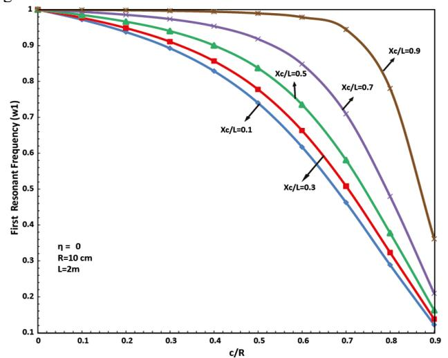
Fig.18. The effect of depth and location of circumferential crack on the first resonant frequency of the shaft.
