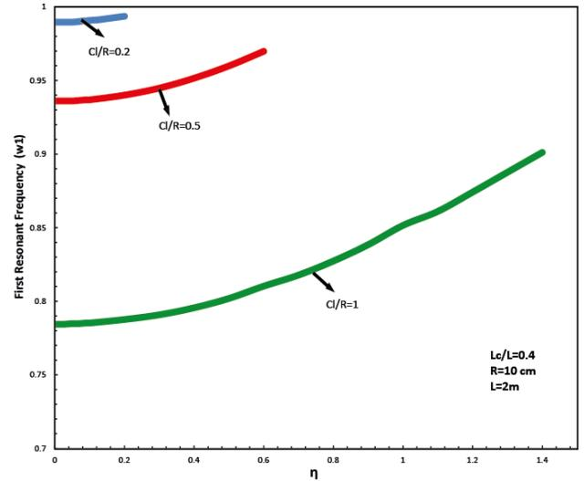
Fig.12. Effects of the energy loss of the longitudinal crack on the frequency response of the shaft for different crack depth ratios. The applied load  $T/T_y = 0.26$  and  $T_y$  the require torque to generate yield stress in the torsional shaft.
