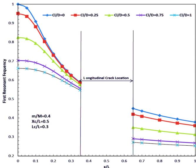
Fig.17. Effects of concentrated mass location on the first resonant frequency of a shaft with longitudinal crack. The concentrated mass value is  $m/M=0.4$ , the crack is located in the middle of the shaft and its length is  $L_c/L=0.3$ .
