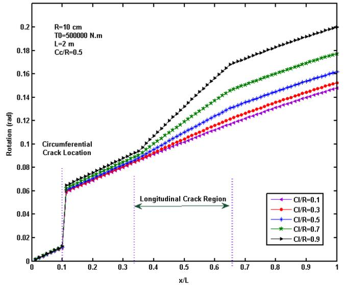
Figure. 20. The indication of rotation along the shaft for a shaft with both circumferential and longitudinal crack with various longitudinal crack depth ratios.
