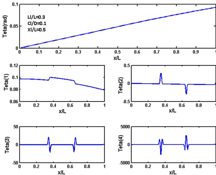
Fig.15. Forced vibration response of a longitudinally cracked shaft and its first four derivate with respect to  $x$ . The crack is located in the middle of the shaft and its length ratio and depth ratio are  $L/L=0.3$  and  $Cl/D=0.1$ .
