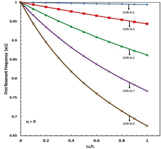
Fig.9. The effect of crack depth on the 1<sup>st</sup> resonant frequency of the shaft for various crack depth ratio.
