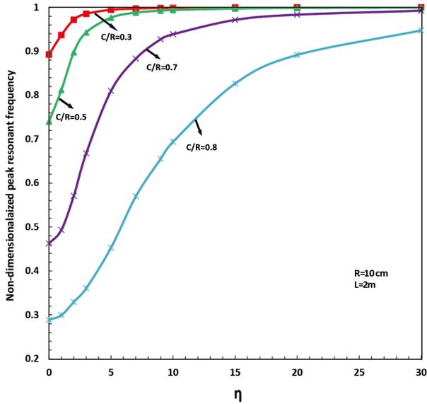
Fig.19. Variation of first non-dimensionalized peak response resonant frequency with energy loss factor
