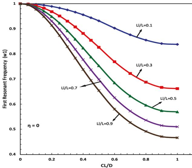
Fig.8. The effect of crack depth on the 1<sup>st</sup> resonant frequency for various crack length ratio.
