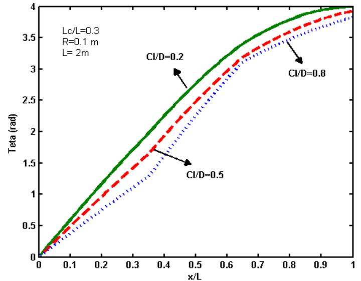
Fig.13. effects of longitudinal crack depth on the 1<sup>st</sup> mode shape of the shaft with crack length  $L_c/L = 0.3$ .
