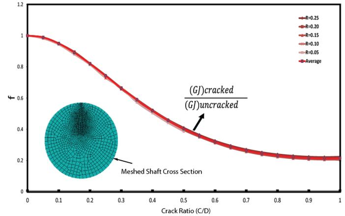
Fig. 3 Torsional rigidity correction factor for a shaft with longitudinal crack
