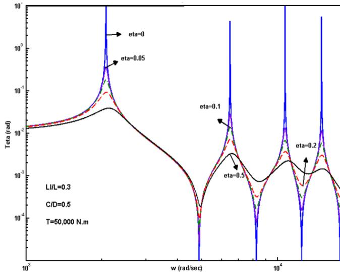
Fig.11. Effects of energy loss on the frequency response of the shaft with longitudinal crack depth  $C/D = 0.5$ , length  $L_c/L = 0.3$  and applied load  $50,000$  N.m.
