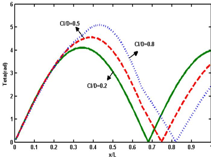
Fig.14. effects of longitudinal crack depth on the 2<sup>nd</sup> mode shape of the shaft with crack length  $L_c/L=0.3$ .
