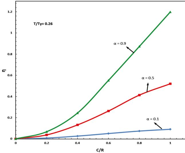
Fig.10. The variation of crack loss factor over a wide range of crack depth for different stress distributions,  $\alpha = 0.1, 0.5$  and  $0.9$ . The load  $T/T_y = 0.26$  and  $T_y$  is the required torque to generate yield stress in the torsional shaft.
