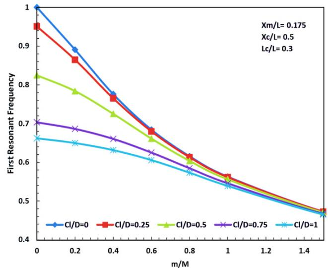
Fig.16. Effects of concentrated mass on the first resonant frequency of a shaft with longitudinal crack, the mass is located at  $X_m/L=0.175$ .  $M$  is denoted as the mass of the shaft.
