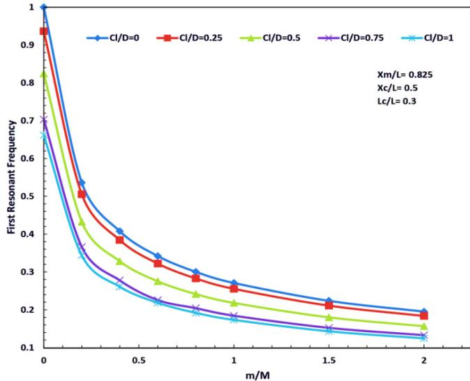
Fig.17. Effects of concentrated mass on the first resonant frequency of a shaft with longitudinal crack, the mass is located at  $X_m/L=0.825$ .
