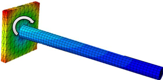
Fig. 2. Finite element model of a shaft with a longitudinal crack subjected to torsion
