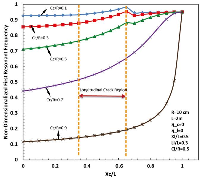
Fig.21. The effect of circumferential crack location and depth on the resonant frequency of a shaft with a longitudinal crack, located in the middle of the shaft.
