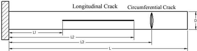
Fig. 7. Schematic model of a shaft with both longitudinal and circumferential cracks.
