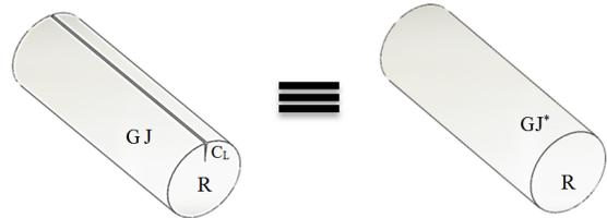
Fig. 4. Equivalent model for a shaft with a longitudinal crack subjected to torsion
