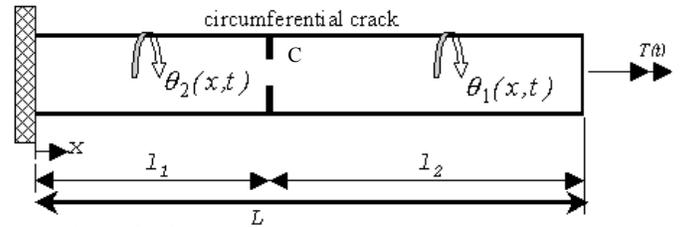
Fig.5 Schematic model of a shaft with a circumferential crack.
