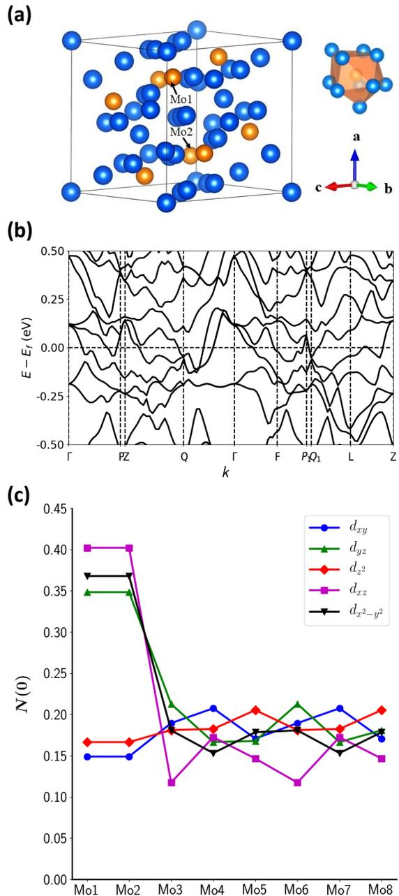
Figure 4: (a) Crystal structure of  $\text{Mo}_8\text{Ga}_{41}$ . (b) Computed band structure plotted along the high-symmetry directions. (c) Computed total density of states at the Fermi level for different Mo sites and different d-orbitals. We observe a clear site-selective phenomena.
