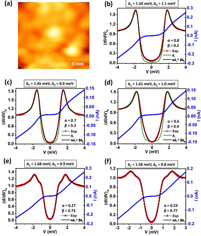
Figure 1: (a) STM topograph image of the sample. (b) (e) Tunneling spectra ( $dI/dV$  vs  $V$  plots) with theoretical fits using Dynes equation showing two gaps measured at 1.9 K. The color dots are experimental data, solid lines show fits with single gap (Green line) and with double gap (Black line).
