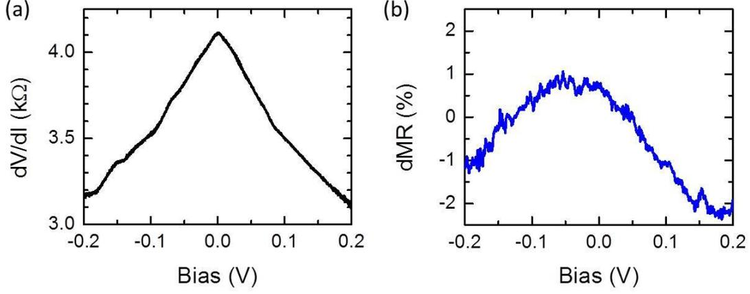
FIG. S4. **Resistance and magnetoresistance of a 2-layer hBN sample.** (a) Differential resistance  $dV/dI$  in the parallel (P) configuration. (b) Differential MR for the same device. No resonant feature can be seen. All data for  $T = 10$  K.
