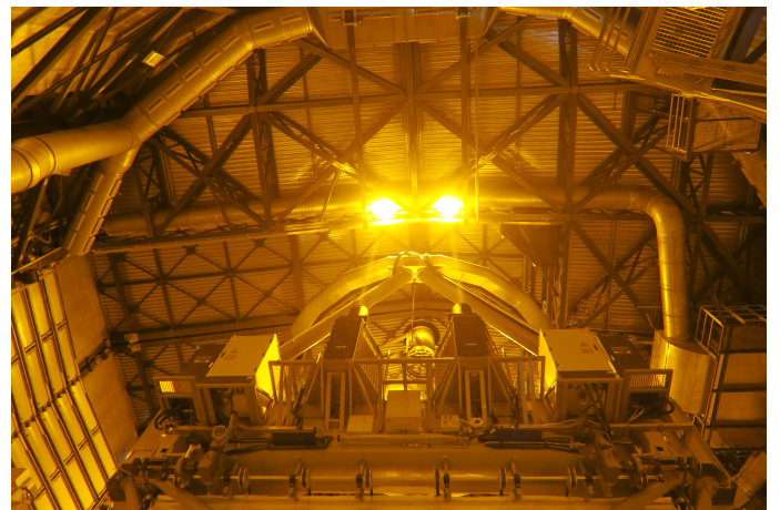
Fig. 3. Picture of the interior of UT4 acquired on 2017-08-15, with the dome closed, the telescope parked, and all four lasers from the 4LGSF propagating. LGS1 and LGS4 are visible in the picture, with their beam hitting the cylindrical structure of an air conditioning duct on the dome roof. The overall glow in the picture is evidence for the high amount of scattering of laser photons by the dome surface. All upper and lower lights in the dome were switched off during the test.
