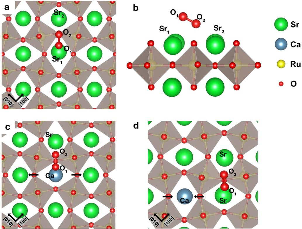
Figure 3: Low coverage of  $\text{O}_2$  adsorbed on (a)-(b) pure and (c)-(d) Ca-doped  $\text{Sr}_3\text{Ru}_2\text{O}_7(001)$ . For Ca-doping, (c) shows the “wide” and (d) the most favored configuration.
