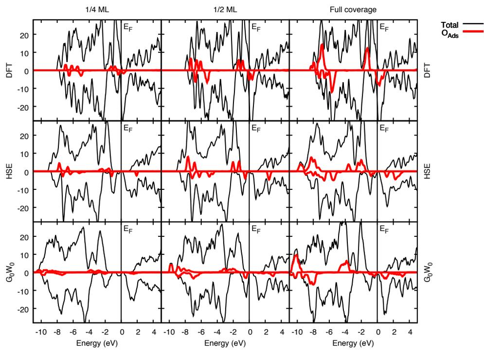
Figure 7: Density of states (DOS) for 1/4 ML, 1/2 ML, and full ML O<sub>2</sub> coverage calculated with the optB86b and HSE06 functional, and the post-DFT many-electron G<sub>0</sub>W<sub>0</sub> method.
