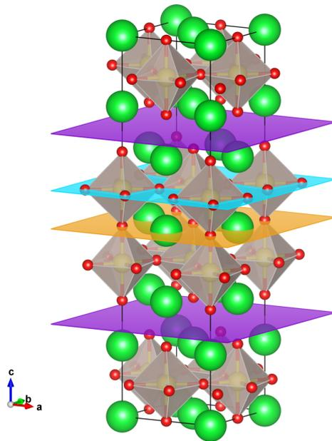
Figure 1: Orthorhombic  $Bbcb$   $Sr_3Ru_2O_7$  crystal structure with the calculated cleavage planes. The rock-salt like (violet) and SrO (orange) cutting planes are both SrO terminated, while the turquoise cleavage plane is  $RuO_2$  terminated. Sr: green, Ru: yellow, O: red.
