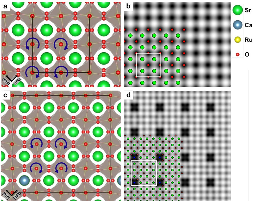
Figure 2: (a):  $c(2 \times 2)$   $\text{Sr}_3\text{Ru}_2\text{O}_7(001)$  surface model cell. (b): corresponding STM simulation ( $\text{Sr}_3\text{Ru}_2\text{O}_7(001)$ ), +0.5 V bias voltage. (c):  $c(4 \times 4)$  Ca-doped  $\text{Sr}_3\text{Ru}_2\text{O}_7(001)$  model cell (6.25% dopant concentration). (d): corresponding STM simulation (Ca-doped  $\text{Sr}_3\text{Ru}_2\text{O}_7(001)$ ), +0.5 V bias voltage.
