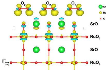
Figure 6: Charge density difference plot at full  $\text{O}_2$  coverage calculated with the optB86b functional. Yellow and turquoise areas indicate charged and depleted areas, respectively.
