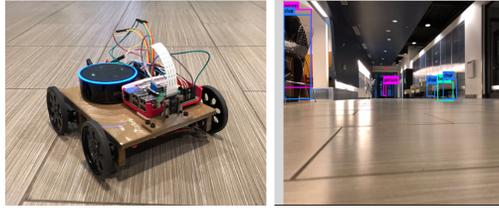
Figure 3. Cloud Chaser and cloud based real time object detection. The right image showcases a screenshot of real time objects being recognized from the Paperspace cloud instance.
