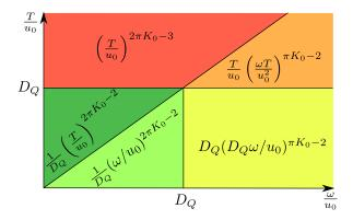
FIG. 2. Scaling behavior of the inverse relaxation time of plasmonic waves due the scattering from QPS in different regimes in the frequency-temperature plane. For each regime, the behavior of  $1/(\tau u_0 y^2)$  is indicated.
