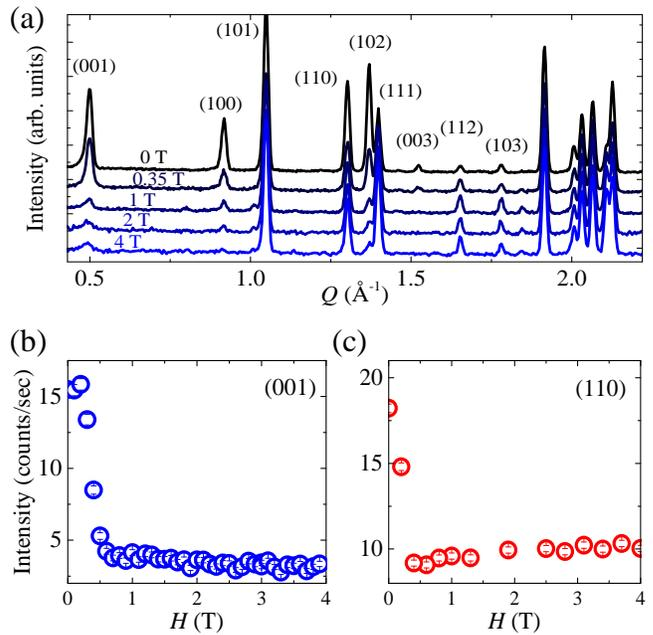
FIG. 6. (a) Waterfall of neutron diffraction patterns collected at 0.5 K under 0, 0.35, 1, 2 and 4 T applied fields. Field dependence of the (b) (001) and (c) (110) peak intensities. All panels are of diffraction data collected using powder samples.
