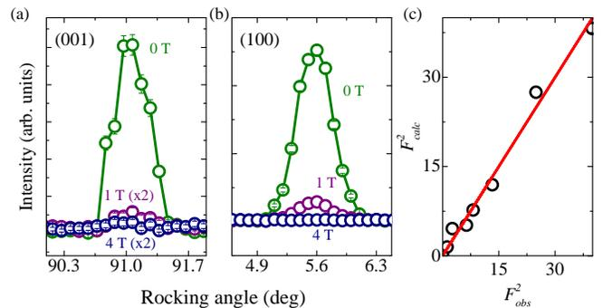
FIG. 7. Single crystal data showing rocking curves on the (a) (001) and (b) (100) magnetic reflections under applied fields of 0, 1 and 4 T. (c) Calculated peak intensities ( $F_{calc}^2$ ) plotted as a function of the observed intensities ( $F_{obs}^2$ ) for Rietveld refinements using the  $P2'_12'_12$  magnetic structure to model the single crystal data collected under a 4 T applied field.
