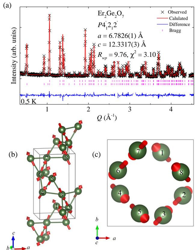
FIG. 5. (a) Rietveld refinement using 0.5 K data and the magnetic structure generated by  $\Gamma_3$ . Refined magnetic structure with Er atoms labeled as described in Fig. 1 viewed along the (b)  $ab$  plane and along the (c)  $c$ -axis.
