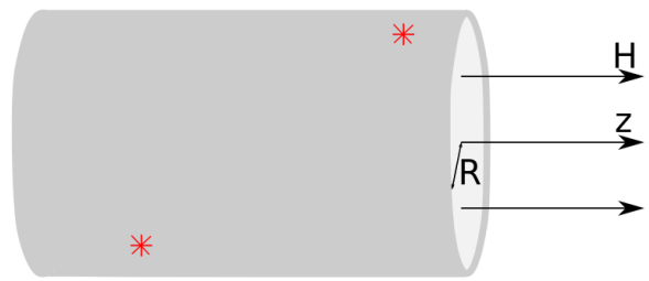
FIG. 4: Thin conducting tube, threaded by magnetic field H . Impurities (shown as stars) are embedded in the tube. Electrons live on the surface of the cylinder.
