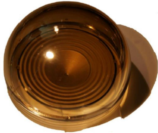
Fig. 1 Left: The ABALONE™ Photosensor schematics. Right: A prototype developed for the IceCube extension project. The inner diameter of the Dome is 10 cm. The base plate and the Dome are made of fused silica, which provides UV sensitivity, as well as a unique level of radio purity. The ABALONE Technology allows fused silica to be used instead of glass without any additional cost to the assembly process.
