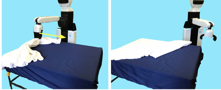
Fig. 10. The HSR following the analytic baseline. It grasps at the highest reachable point and pulls in the direction of the yellow arrow, improving coverage.
