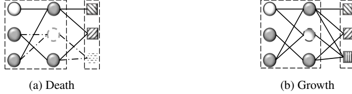
Figure 4: (a) The third abstraction is not good enough and it dies along with the structure it is connected to. (b) The third one is new abstraction produced by a new structure.
