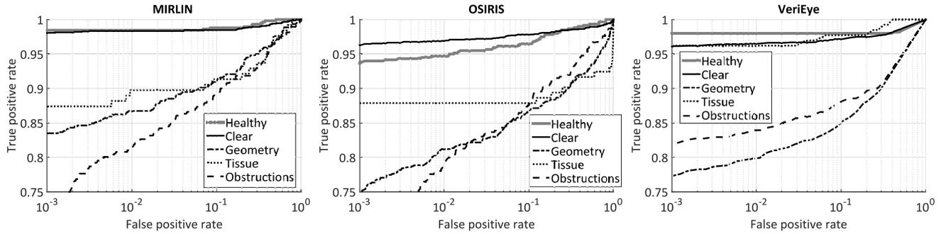
Figure 2. Receiver operating characteristics (ROC) for MIRLIN (left), OSIRIS (middle) and VeriEye (right) iris recognition methods.
