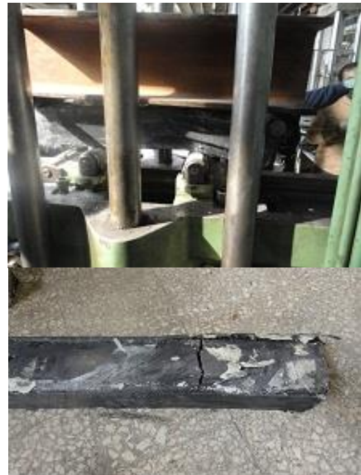
Fig. 7. Flexural weakness of the beams
