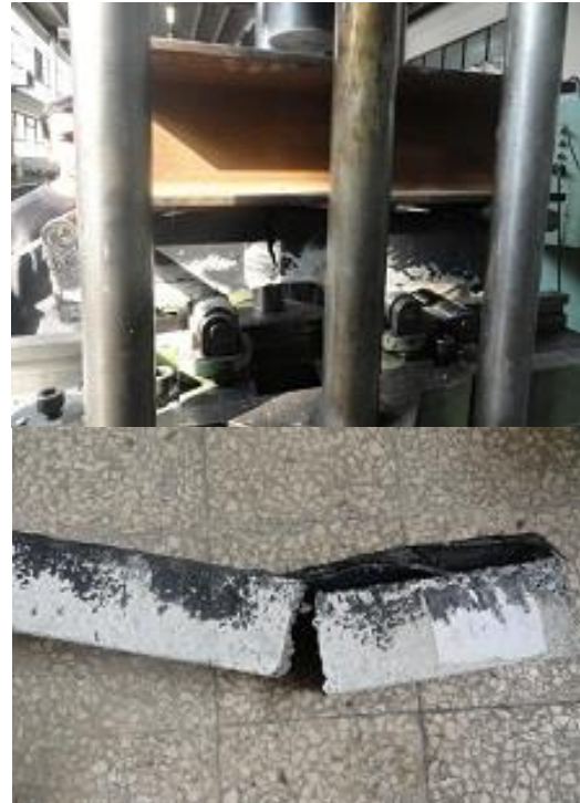
Fig. 6. Strong bond between the concrete and the FRP sheet
