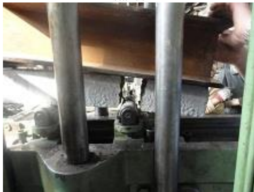
Fig. 5. Premature bond- failure of FRP sheet
