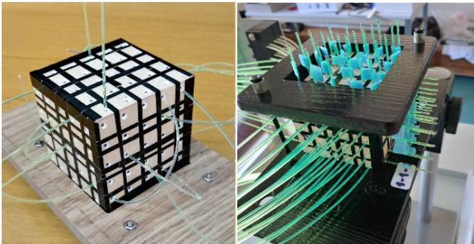
Figure 2: The array of 125 cubes with 3D fiber readout. Right photo shows the array with 75 fibers mounted for the beam test.
