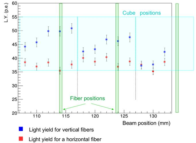
Figure 5: Light yields for horizontal and vertical fibers vs beam position. Also vertical fibers and cube coordinates are shown at the horizontal scale.
