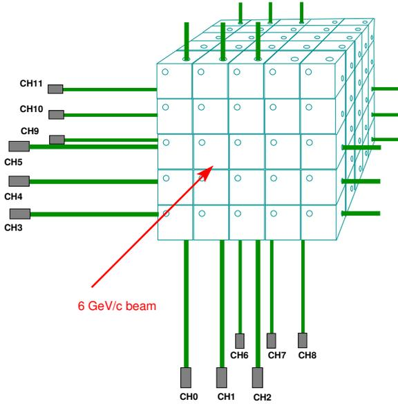
Figure 3: Readout of WLS fibers by the digitizer, and channel labeling. Inactive fibers are not shown.
