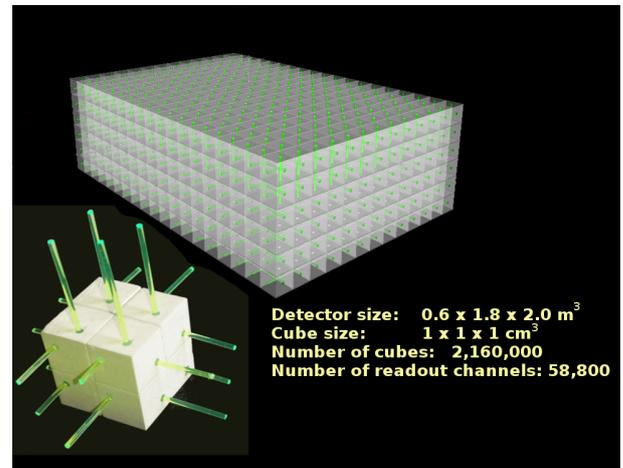
Figure 1: Schematic view of the superFGD conceptual design. An array of  $2 \times 2 \times 2$  scintillator cubes illustrates the 3D readout by Wave Length Shifting (WLS) fibers.
