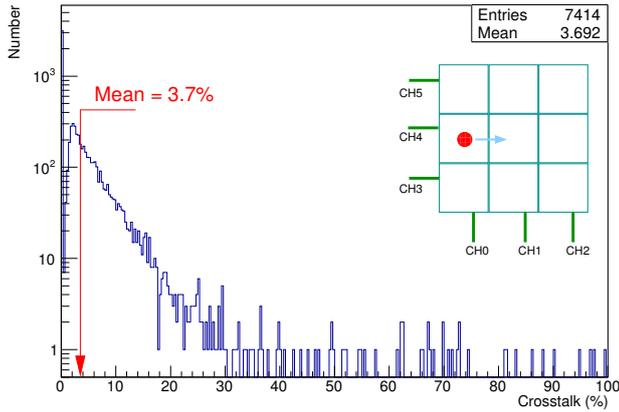
Figure 6: Crosstalk from the cube ch0/ch4 into the cube ch1/ch4. Beam hits the central part of the ch0/ch4 cube.
