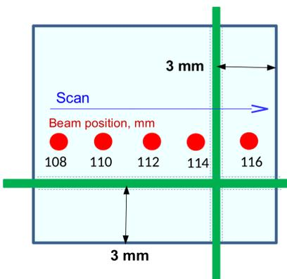
Figure 4: Beam scan across a single cube. Fiber positions (in green) are shown relative to the beam hit points (in red).
