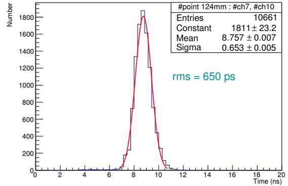
Figure 8: Charge and time spectra for a single cube. Charge signal is a sum from two fibers, the time is an average time between two fibers.
