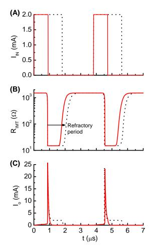
**Fig. 9. Simulated waveform for current-clamp VO<sub>2</sub> neuron**. (A) Input current, (B) VO<sub>2</sub> resistance and (C) Output current. The red solid lines and black dot lines are two different inputs that result in the same firing patterns. The extra current inputs are not being integrated to the capacitor due to the existence of post refractory period. This property directly mimics the biological neuron.
