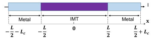
**Fig. 6. Full schematic of an IMT device with length L between two metal contacts.** The device is discretized into segment of dx, etch with its own temperature and resistivity. Heat conduction is along x direction while convective heat loss through the side wall.
