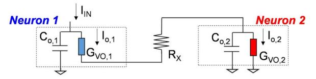
Fig. 13. VO<sub>2</sub> monosynaptic neuron circuit.
