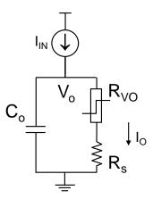
Fig. 7. The complete VO<sub>2</sub> neuron circuit. The whole circuit contains three elements: a capacitor as well as the VO<sub>2</sub> device with a sensing resistor in series. The output current is sensed by the sensing resistor. The voltage at the capacitor node is denoted as  $V_0$ . It is also the input node for the injected current.
