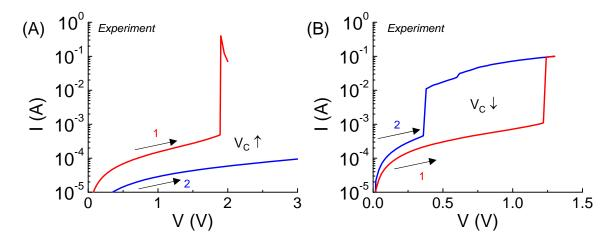
**Fig. 2.** VO<sub>2</sub> device under excessive DC stress experiencing non-reversible change in critical transition voltage. Two consecutive sweeps are applied to the VO<sub>2</sub> device with the first sweep stresses the device. (A) Increase in V<sub>c</sub> is caused by an increase of HRS resistance,  $+\Delta R$ . (B) Reduction in V<sub>c</sub> is the indication of a drop in HRS resistance,  $-\Delta R$ .
