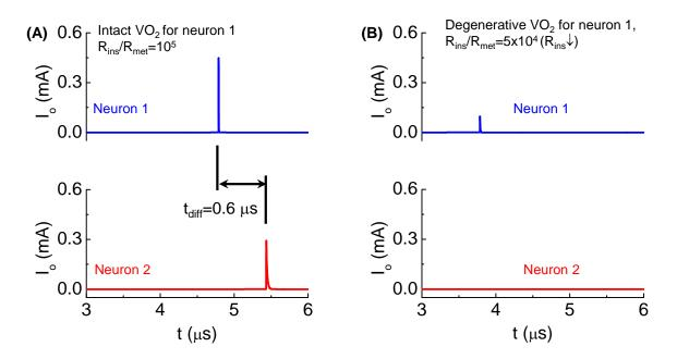
Fig. 14. Demonstration of degenerative Neuron 1 leading to the failed signal reception for Neuron 2 in a monosynaptic circuit. (A) Output current as a function of time shows the spike events for the intact case. (B) Premature spike in Neuron 1 when its HRS resistance is reduced and Neuron 2 fails to spike.
