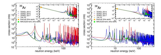
FIG. 20. Excitation functions of the  $^{36,38}$ Ar $(n,\gamma)$  reaction calculated with the Hauser-Feshbach codes indicated. The experimental values of the thermal cross section and of the MACS(30 keV) determined in this work are shown. The excitation functions are matched to the thermal cross sections measured in this work.
