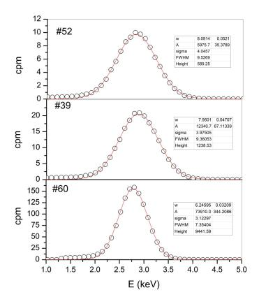
FIG. 14. Energy spectra (in counts per minute) and gauss fit of  $^{37}$ Ar measurements by low-level counting (LLC). The peak energy correspond to the 2.82 keV K-capture decay energy of  $^{37}$ Ar.
