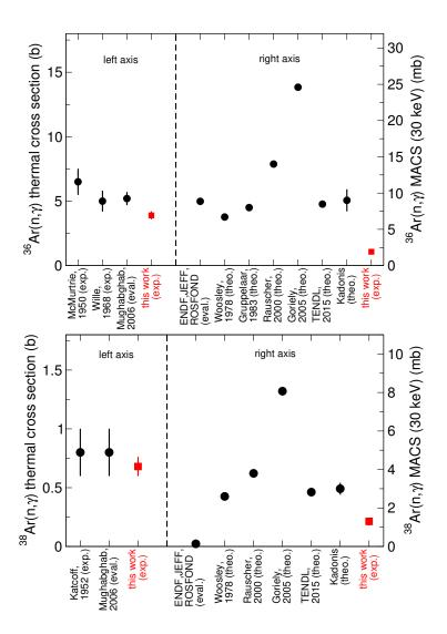
FIG. 21. Comparison of the <sup>36</sup>Ar (top) and <sup>38</sup>Ar (bottom) thermal and Maxwellian Average (30 keV) cross sections measured in this work (red squares) to measured (thermal) and theoretical data (black circles). Numerical values are listed in Table II (main paper).
