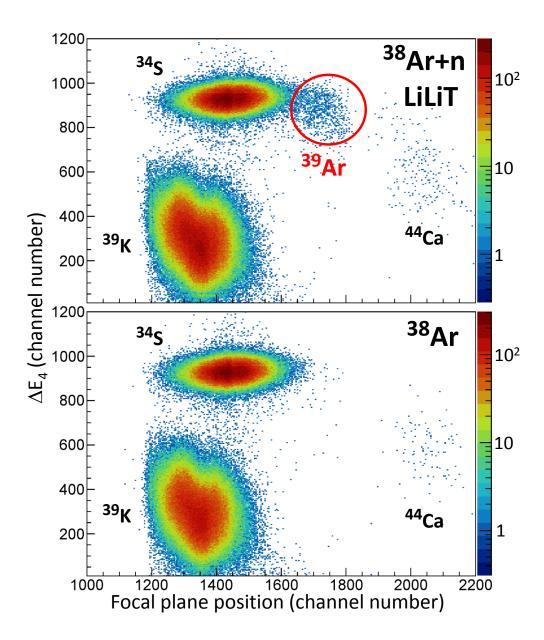
FIG. 3. Identification spectrum of <sup>39</sup>Ar ions in the detector measured for the LiLiT irradiated <sup>38</sup>Ar gas (top) and for non-irradiated <sup>38</sup>Ar gas (bottom). The horizontal axis represents dispersion along the focal plane and the vertical axis a differential energy loss signal measured in the fourth anode of the focal-plane ionization chamber [36].
