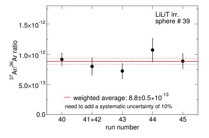
FIG. 12. Repeated measurements of the  $^{37}\mathrm{Ar}/^{36}\mathrm{Ar}$  ratio for the LiLiT irradiated sphere (#39). See Table IV for numerical results.
