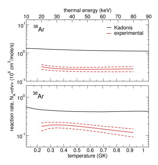
FIG. 4. (Color online) Comparison of the  $^{36}$ Ar (top) and  $^{38}$ Ar (bottom)  $(n, \gamma)$  reaction rates  $(N_A \langle \sigma v \rangle)$  extracted from this work (red) to the Kadonis [49] recommended values (black). The dashed curves encompass the estimated  $1\sigma$  uncertainty.
