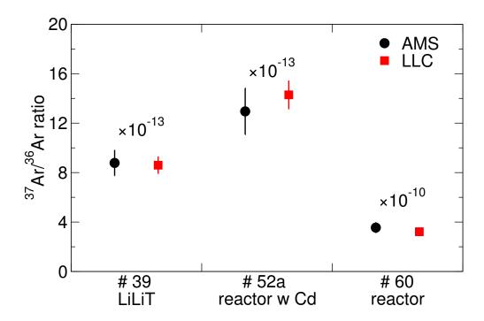
FIG. 2. (Color online) Comparison of the <sup>37</sup>Ar/<sup>36</sup>Ar ratio (at the end of irradiation) measured by AMS (black) and LLC (red).
