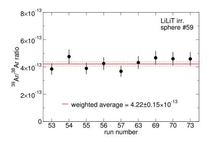
FIG. 16. Repeated measurements of the  $^{39}\mathrm{Ar}/^{38}\mathrm{Ar}$  ratio for the LiLiT irradiated sphere (#59). See Table VIII for numerical results.
