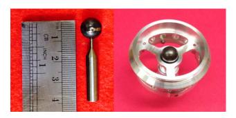
FIG. 6. Ti sphere used as container for the pressurized  ${}^{A}$ Ar gas for irradiation (left), and the sphere target holder for irradiation at SARAF-LiLIT (right).
