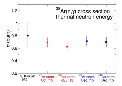
FIG. 19. Comparison of the measured  $^{38}$ Ar thermal cross section using external  $^{198}$ Au and internal  $^{41}$ Ar neutron monitoring.
