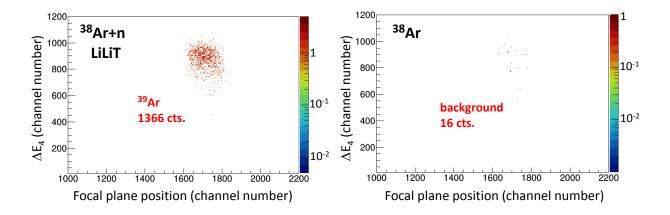
FIG. 11. Two-dimensional spectra of  $\Delta E_4$  vs. focal plane position gated on the <sup>39</sup>Ar region-of-interest in the time-of-flight,  $\Delta E_2$  and  $\Delta E_3$  detector parameters.
