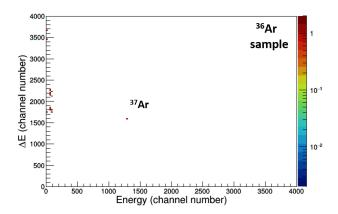
FIG. 10. Same as Fig. 7 for a non irradiated  $^{36}$ Ar (blank). One  $^{37}$ Ar count detected for this sample over 6.5 hours, likely due to a memory effect in the ion source, corresponds to a concentration  $^{37}$ Ar/ $^{36}$ Ar=9 × 10<sup>-16</sup>.
